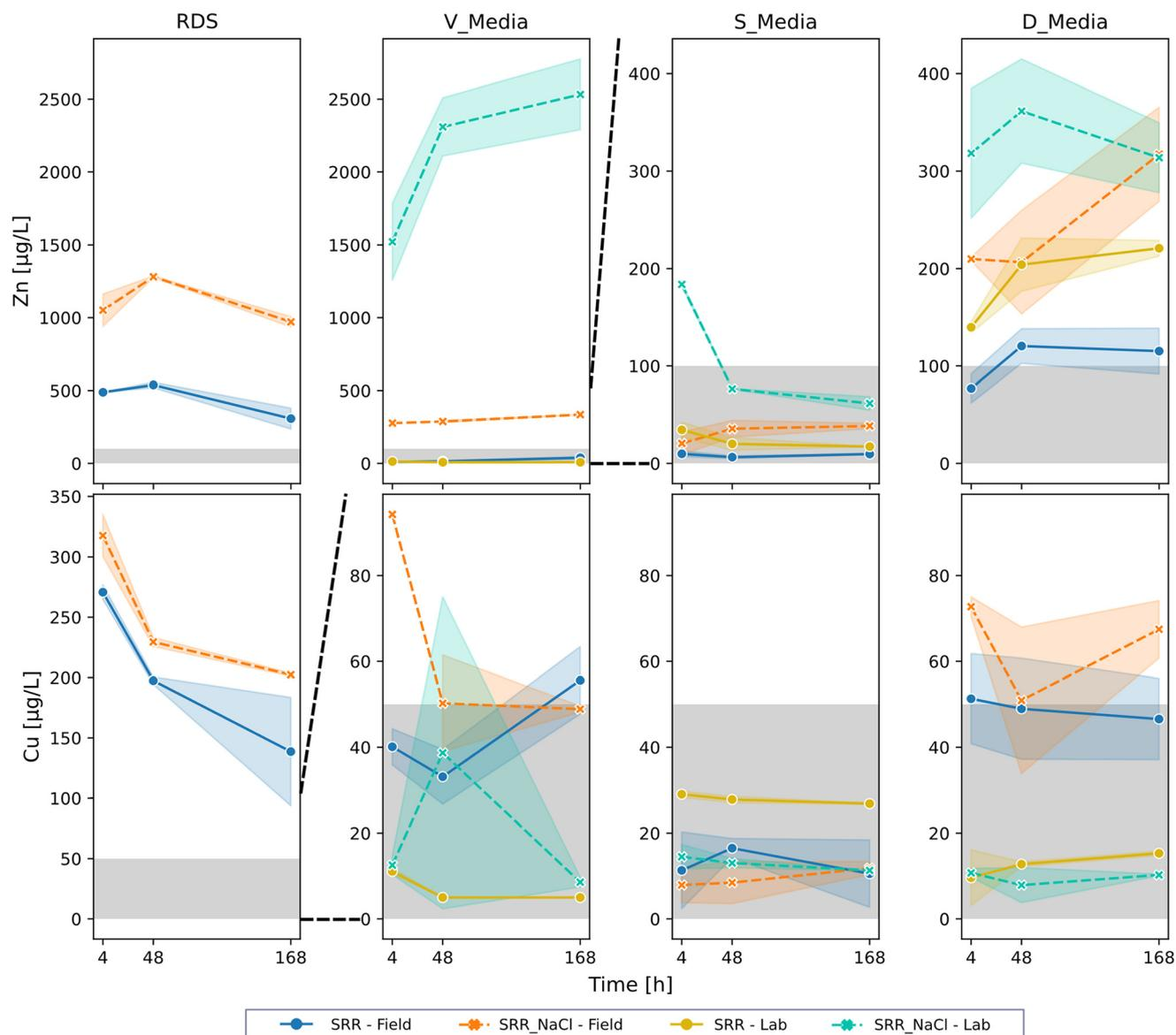
**Fig. 1** Time series of the mean dissolved Zn and Cu concentrations in the leachate of the different media; the gray area indicates concentrations below the initial concentration of the synthetic road runoffs; values above the grey area imply leaching; the standard deviation is represented by the colored shaded area.
