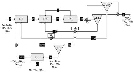
Fig. 1 WWTP Katwoude, adapted from Meijer et al.<sup>20</sup> Unit processes are indicated in grey: R1 = mixed non-aerated selector, R2 = completely mixed anoxic reactor, R3 = aerated carrousel reactor, CL12, CL34 = four clarifiers were operated in pairs. fd1, fd2, fd3 = flow dividers, TH = sludge thickener and CE = centrifuge. The black boxes refer to the name of the streams. The measured variables are indicated by name at their respective positions
