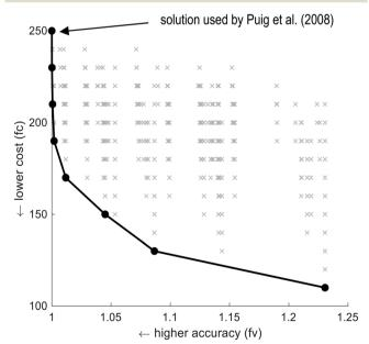
Fig. 4 Pareto optimal solutions for the setup of Puig et al.<sup>22</sup> determined using the experimental procedure of Le et al. 17 and expressed in terms of accuracy and costs. The line with the filled black circles denotes the Pareto-optimal front. 'x' = a solution.
