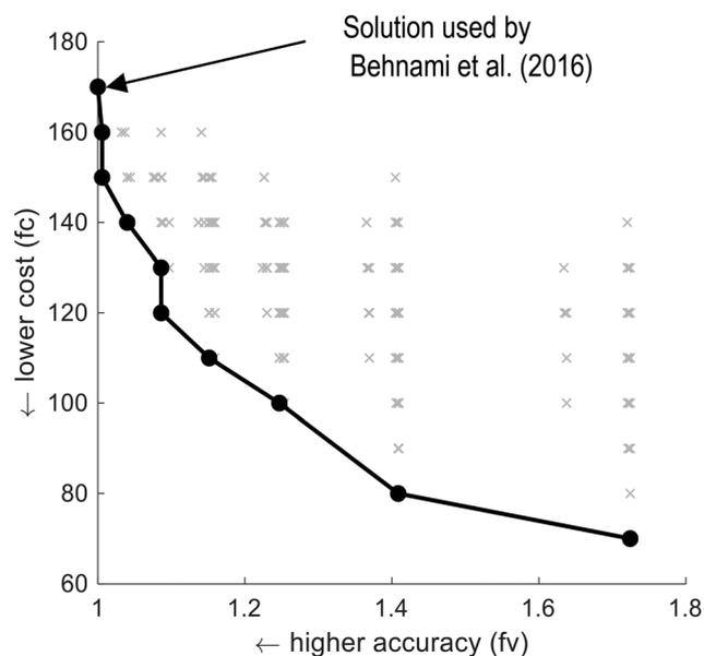
Fig. 8 Pareto optimal solutions for the setup of Behnami *et al.*<sup>19</sup> determined using the experimental procedure of Le *et al.*<sup>17</sup> and expressed in terms of accuracy and costs. The line with the filled circles denotes the Pareto-optimal front. 'x' = a solution.
