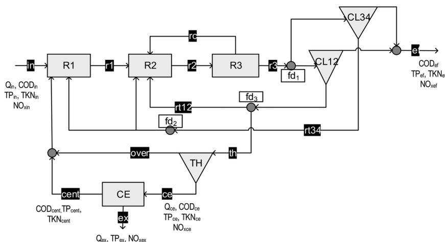
**Fig. 1** WWTP Katwoude, adapted from Meijer *et al.*<sup>20</sup> Unit processes are indicated in grey: R1 = mixed non-aerated selector, R2 = completely mixed anoxic reactor, R3 = aerated carousel reactor, CL12, CL34 = four clarifiers were operated in pairs.  $fd_1$ ,  $fd_2$ ,  $fd_3$  = flow dividers, TH = sludge thickener and CE = centrifuge. The black boxes refer to the name of the streams. The measured variables are indicated by name at their respective positions.
