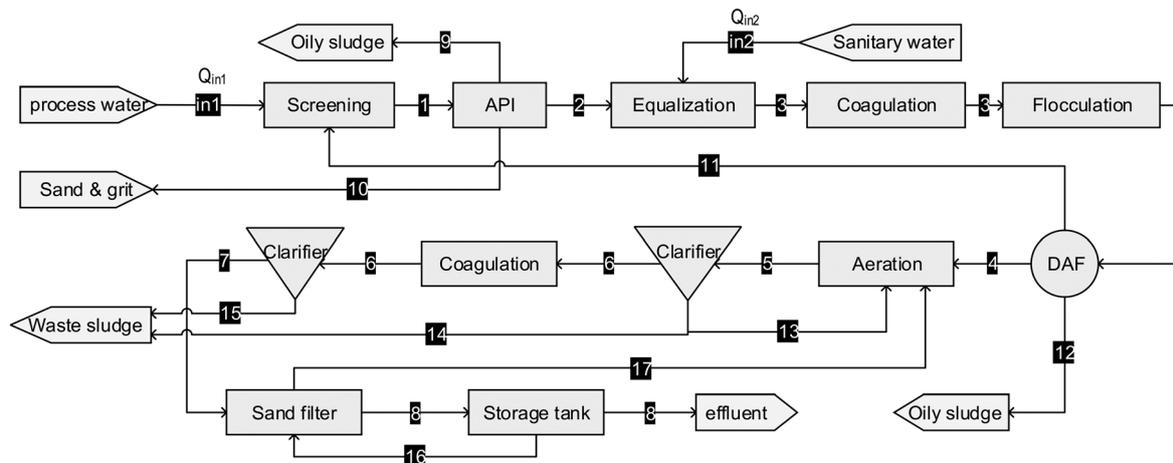
Fig. 7 Flow diagram of the Tabriz petrochemical WWTP, Iran.<sup>19</sup> Measured variables are presented.
