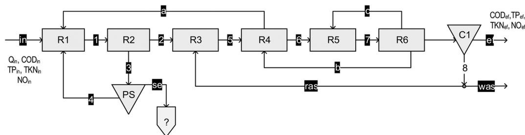
Fig. 3 Flow diagram of the Deventer WWTP, The Netherlands (adapted from Puig *et al.*<sup>22</sup>). R1 and R2 = two anaerobic reactors, R3 = a contact tank, R4 = an anoxic reactor, R5 = an alternatively aerated reactor, R6 = aerated reactor, C1 = six secondary settlers (in parallel) and PS = stripping reactor. Measured variables are indicated.
