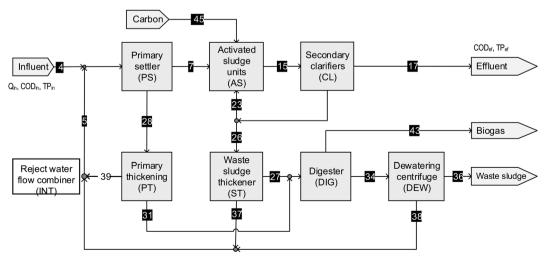
Fig. 5 Flow diagram of the Houtrust WWTP, The Netherlands, adapted from Meijer et al.<sup>21</sup> Measured variables are indicated.
