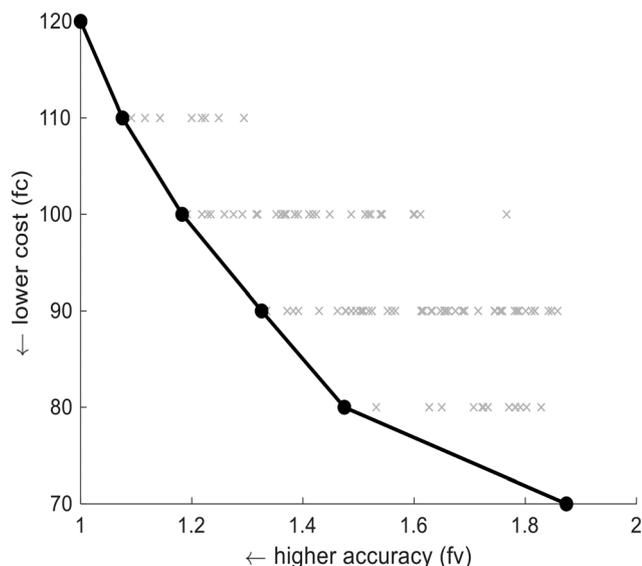
Fig. 2 Pareto optimal solutions for the setup of Meijer *et al.*<sup>20</sup> determined by the experimental procedure of Le *et al.*<sup>17</sup> and expressed in terms of accuracy and costs. The line with the filled circles (black) denotes the Pareto-optimal front. 'x' = a solution.
