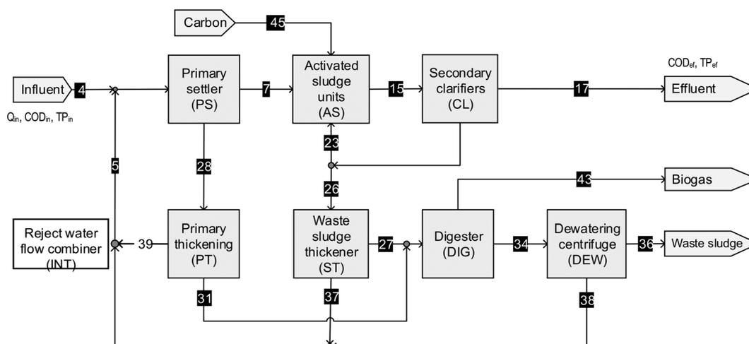
Fig. 5 Flow diagram of the Houtrust WWTP, The Netherlands, adapted from Meijer *et al.*<sup>21</sup> Measured variables are indicated.
