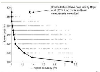
Fig. 6 Pareto optimal solutions for the setup of Meijer et al.<sup>21</sup> determined using the experimental procedure of Le et al. 17 and expressed in terms of accuracy and costs. The line with the filled grey circles denotes the Pareto-optimal front. 'x' = a solution
