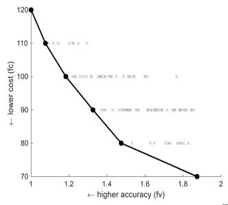
Fig. 2 Pareto optimal solutions for the setup of Meijer et al.<sup>20</sup> determined by the experimental procedure of Le et al. 17 and expressed in terms of accuracy and costs. The line with the filled circles (black) denotes the Pareto-optimal front, 'x' = a solution.
