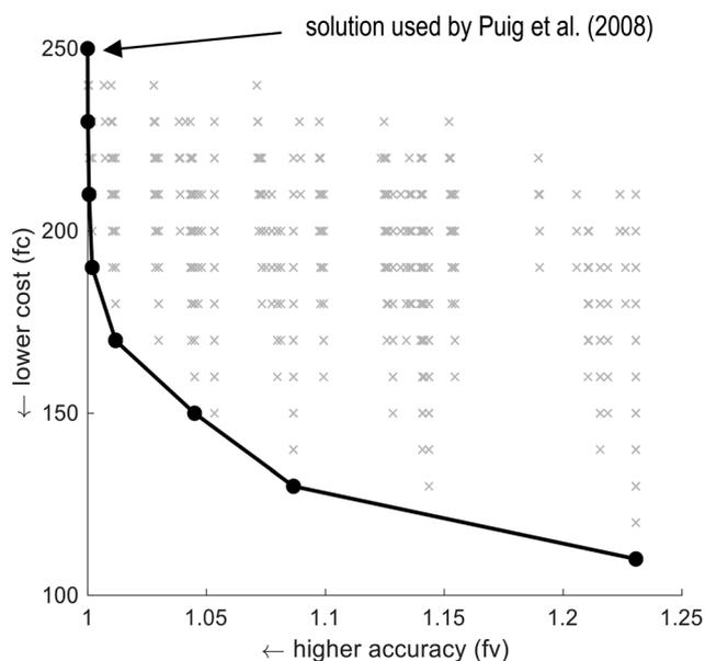
**Fig. 4** Pareto optimal solutions for the setup of Puig *et al.*<sup>22</sup> determined using the experimental procedure of Le *et al.*<sup>17</sup> and expressed in terms of accuracy and costs. The line with the filled black circles denotes the Pareto-optimal front. 'x' = a solution.
