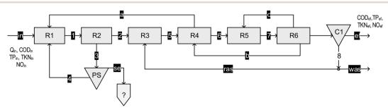
Fig. 3 Flow diagram of the Deventer WWTP, The Netherlands (adapted from Puig et al.<sup>22</sup>). R1 and R2 = two anaerobic reactors, R3 = a contact tank, R4 = an anoxic reactor, R5 = an alternatively aerated reactor, R6 = aerated rector, C1 = six secondary settlers (in parallel) and PS = stripping reactor. Measured variables are indicated.
