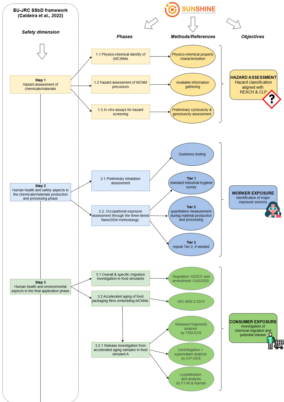
Fig. 2 Graphical representation of the SUNSHINE methodology applied to address the safety aspects (as identified by the EU-JRC SSbD framework) of the BNT-CEO-based LDPE case study. Ellipses display the methods adopted within each phase of the assessment, in agreement with standard or recommended procedures.
