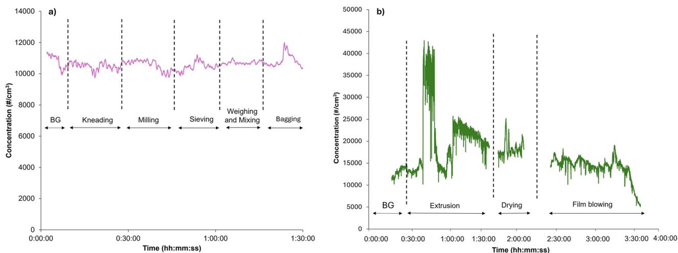
Fig. 7 Particle number concentration during a) BNT-CEO synthesis (ES1) and b) LDPE(BNT-CEO) production and processing (ES2).
