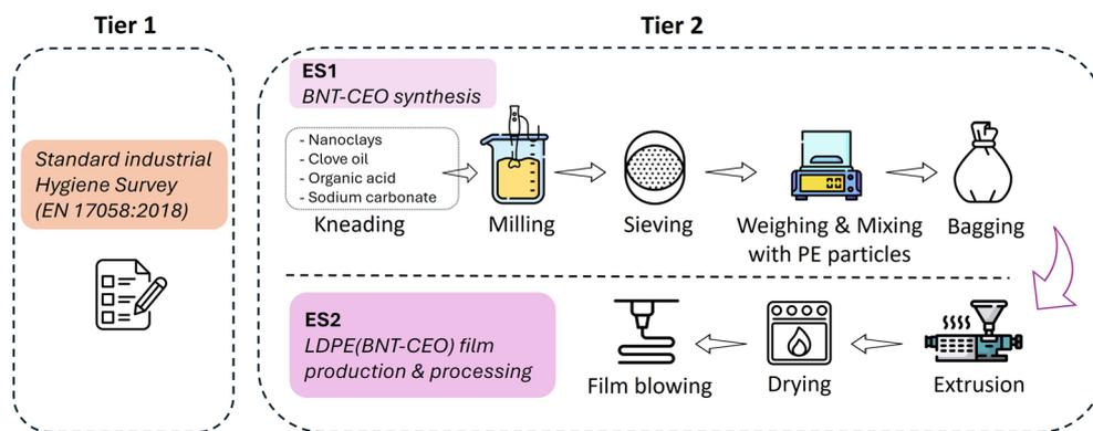
Fig. 3 Schematic of the tiered methodology approach applied to assess the occupational safety and health (OSH) aspects of the BNT-CEO synthesis (ES1) and the LDPE(BNT-CEO) film production and processing (ES2).
