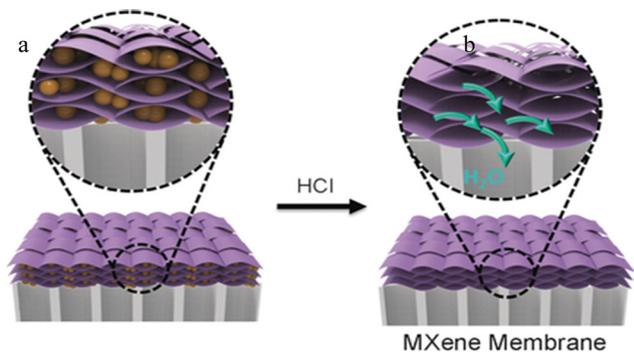
Fig. 7 (a) 2D MXene nanosheets based membrane with colloidal Fe(OH)<sub>3</sub> (yellow spheres). (b) Hydrochloric acid solution (HCl) treatment to remove the Fe(OH)<sub>3</sub> nanoparticles from the synthesized MXene. Reproduced from ref. 45 with permission from Wiley, copyright 2017.
