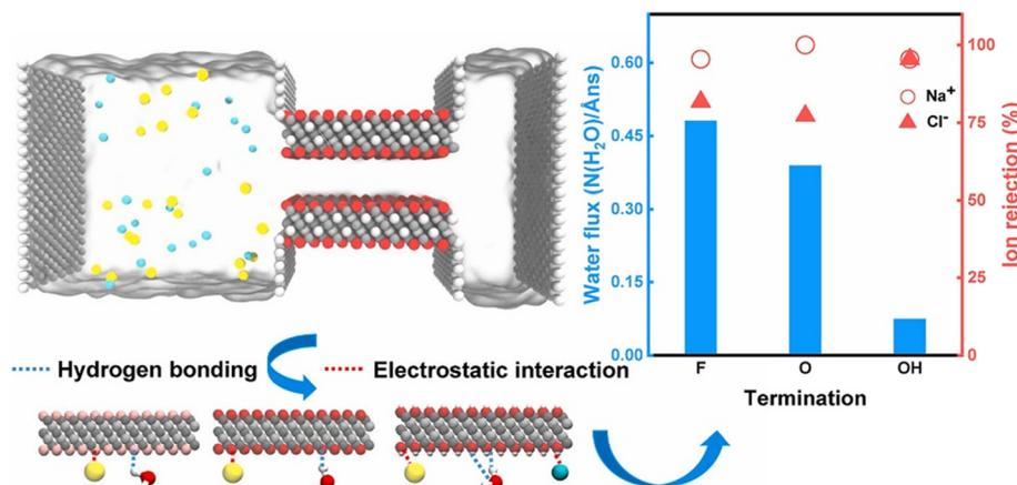
Fig. 2 (Left) Simulation model for the desalination process. (Right) Water flux through nanochannels functionalized with different MXene-based membrane termination groups.<sup>44</sup> Reproduced from ref. 44 with permission from Elsevier, copyright 2022.
