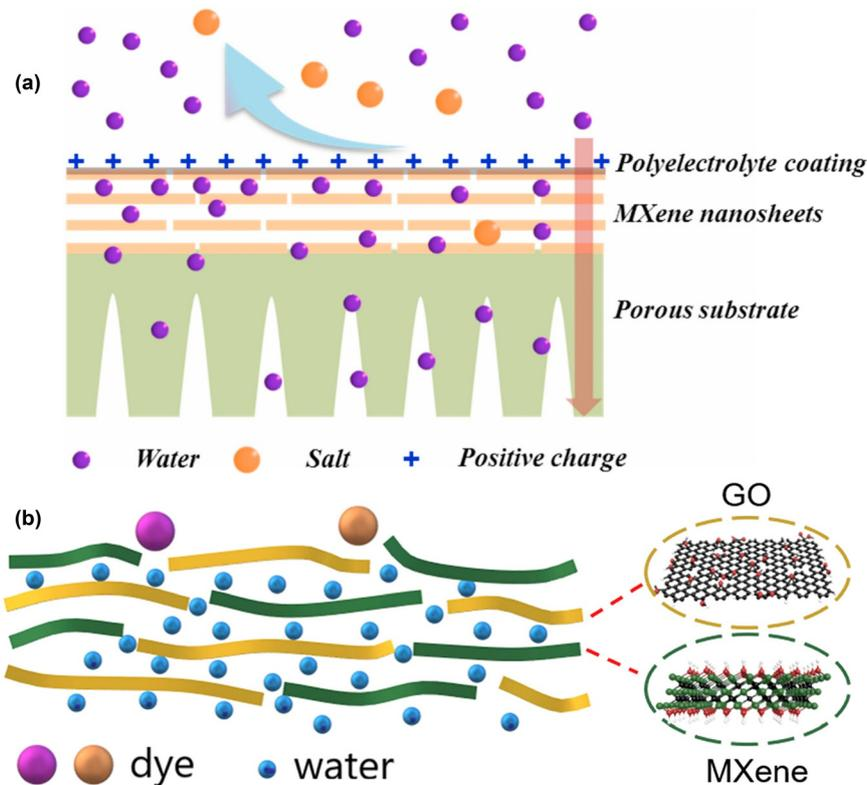
**Fig. 8** (a) Laminar stacking of MXene nanosheet based membrane with a polyelectrolyte surface coating (SC). Reproduced from ref. 52 with permission from Elsevier, copyright 2021. (b) GO/MXene composite membranes were fabricated for water treatment. Reproduced from ref. 125 with permission from Elsevier, copyright 2020.
