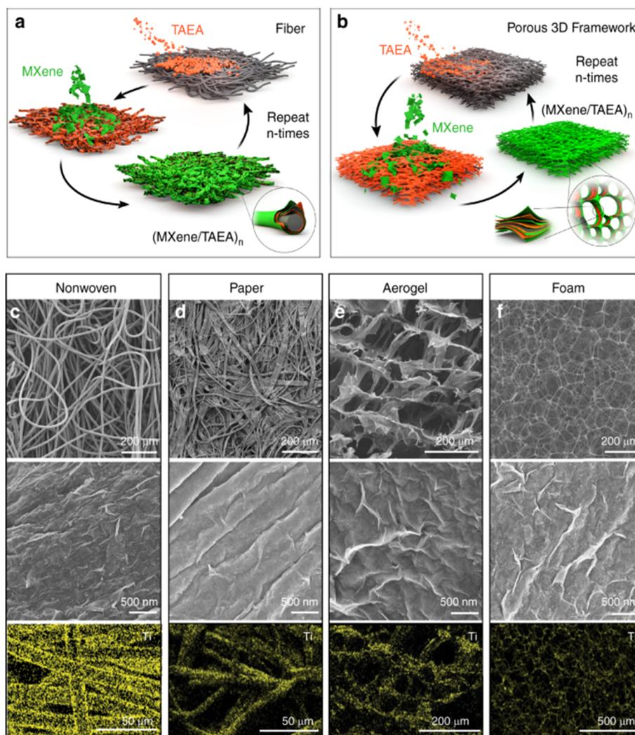
Fig. 4 Layer-by-layer (LbL) assembly of MXene/tris(2-aminoethyl)amine, (TAEA)<sub>n</sub> layers on (a) fibres and (b) foams. Physicochemical analysis of MXenes layers coated on different samples of (c) nonwoven, (d) cellulose paper, (e) cellulose nanofibers (CNF) and (f) melamine foam. Reproduced from ref. 129 under a Creative Commons CC BY License.
