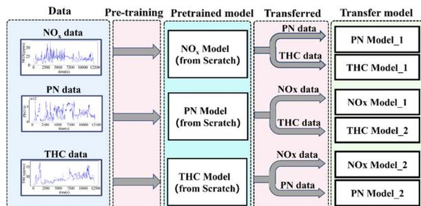
Transfer learning for transient NO<sub>x</sub>, PN and THC emission prediction of non-road diesel engines based on NRTC experiments
