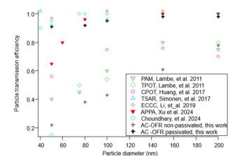
Fig. 5 Comparative particle transmission efficiency between the AC-OFR and similar OFRs reported in the literature.
