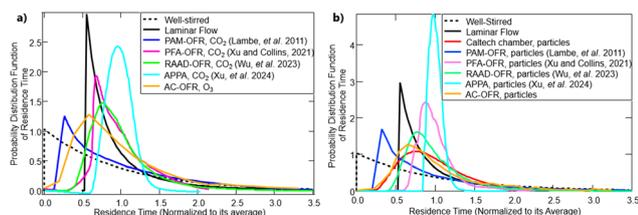
Fig. 4 Probability Distribution Function (PDF) of the residence time for the PAM-OFR (Lambe *et al.*, 2011), PFA-OFR (Xu and Collins, 2021), RAAD-OFR (Wu *et al.*, 2023), APPA (Xu *et al.*, 2024) and the AC-OFR for (a) gases and (b) particles.
