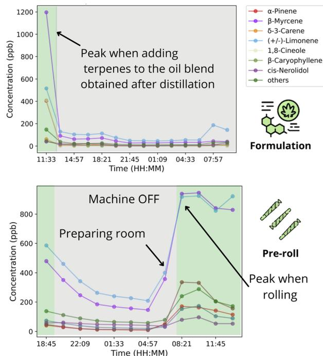
**Fig. 4** Time series of the formulation and pre-roll activities, which caused spikes in concentration. In formulation, the peak is a result of adding terpenes to the vape mix being prepared. In the pre-roll, just by prepping the room bringing raw material inside cause an increase in concentration. When the pre-roll machine is in operation, concentration reaches a peak.
