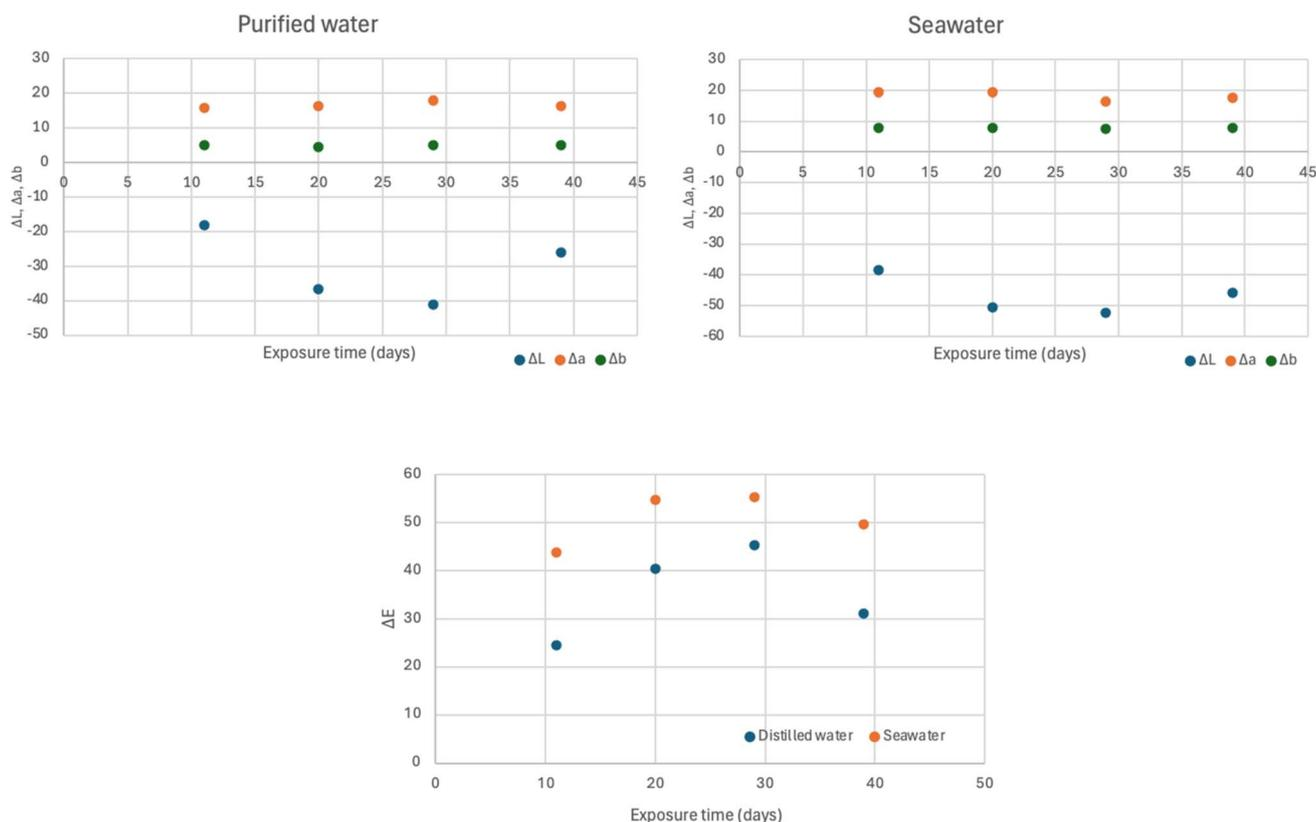
Fig. 2 Differences in color between the original glitter (blue) and aged glitter at different exposure times. (a) Differences in  $\Delta L$ ,  $\Delta a$  and  $\Delta b$  in purified water, (b) differences in  $\Delta L$ ,  $\Delta a$  and  $\Delta b$  in seawater and (c) global differences ( $\Delta E$ ).
