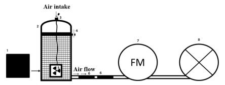
Fig. 1 Scheme of apparatus used for measurement of  $K_{TA}$  of AAs; 1- textile pieces before wrapping to the chamber mesh (Fig S1†), 2- glass chamber with a ground joint lid, mesh and airtight seal, 3- steel capillary pierced through a septum for air intake, 4- metal clamp, 5- small fan, 6two glass tubes filled with Tenax adsorbent, in series, 7- air mass flow meter, 8- low volume air pump.
