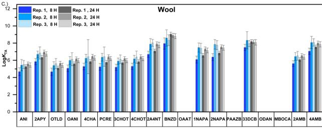
Fig. 2  $K_{TA}$  (L kg<sup>-1</sup>, log-transformed) of aromatic amines for three types of textiles — (A) polyester, (B) cotton, and (C) wool. Data were collected from two experiments performed at two different air flow conditions (thus differing in experiment duration of 8 hours and 24 hours); each experiment was conducted in triplicate.
