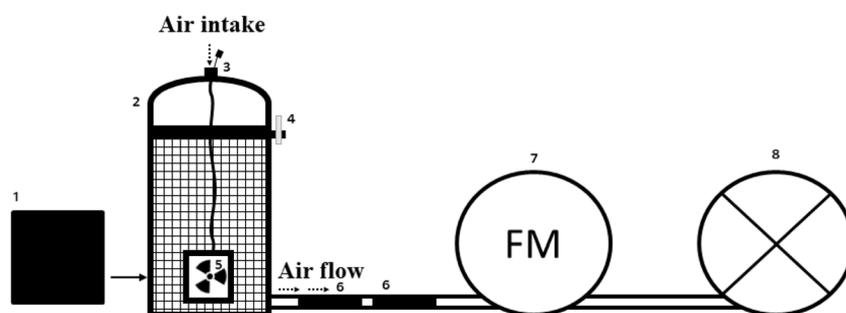
Fig. 1 Scheme of apparatus used for measurement of  $K_{TA}$  of AAs; 1- textile pieces before wrapping to the chamber mesh (Fig S1†), 2- glass chamber with a ground joint lid, mesh and airtight seal, 3- steel capillary pierced through a septum for air intake, 4- metal clamp, 5- small fan, 6- two glass tubes filled with Tenax adsorbent, in series, 7- air mass flow meter, 8- low volume air pump.
