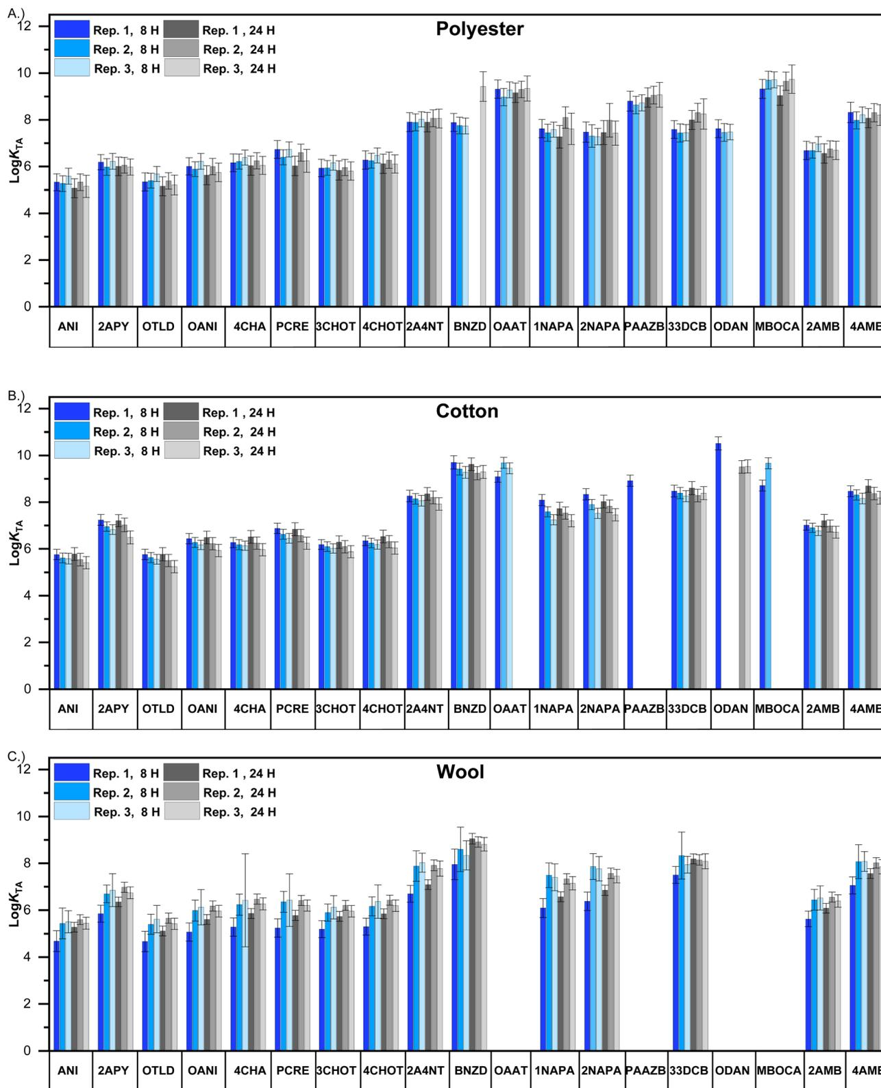
Fig. 2  $K_{TA}$  ( $\text{L kg}^{-1}$ , log-transformed) of aromatic amines for three types of textiles — (A) polyester, (B) cotton, and (C) wool. Data were collected from two experiments performed at two different air flow conditions (thus differing in experiment duration of 8 hours and 24 hours); each experiment was conducted in triplicate.
