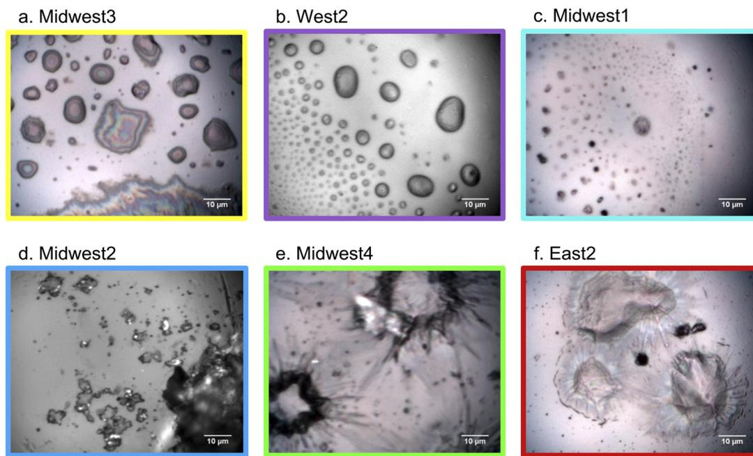
Fig. 2 Representative optical microscopy images of the glass substrate surfaces using a 100 $\times$  objective (0.9 N.A.) on an Olympus microscope to characterize deposition from select kitchen samples: (a) Midwest3, (b) West2, (c) Midwest1, (d) Midwest2, (e) Midwest4, (f) East2.
