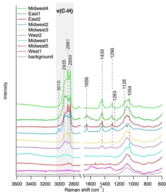
Fig. 6 Raman spectra from kitchens collected over 3 weeks. The gray box highlights the C–H stretching region. Note that the East1 Raman spectrum is the same as shown in Fig. 4. The peak around  $1100\text{ cm}^{-1}$  is from the glass substrate and indicated with an asterisk.
