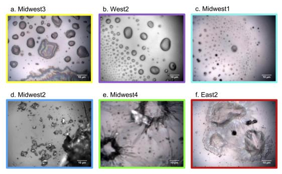
Fig. 2 Representative optical microscopy images of the glass substrate surfaces using a 100× objective (0.9 N.A.) on an Olympus microscope to characterize deposition from select kitchen samples: (a) Midwest3, (b) West2, (c) Midwest1, (d) Midwest2, (e) Midwest4, (f) East2.
