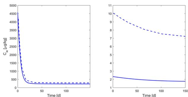
Fig. 3 Exemplary visualization of the simulated sulfamethoxazole (left) and trimethoprim (right) concentration under sterilized conditions in soil water ( $C_w$ ) without extraction (solid blue) and as it would be observed in the extracted fraction (dashed blue).
