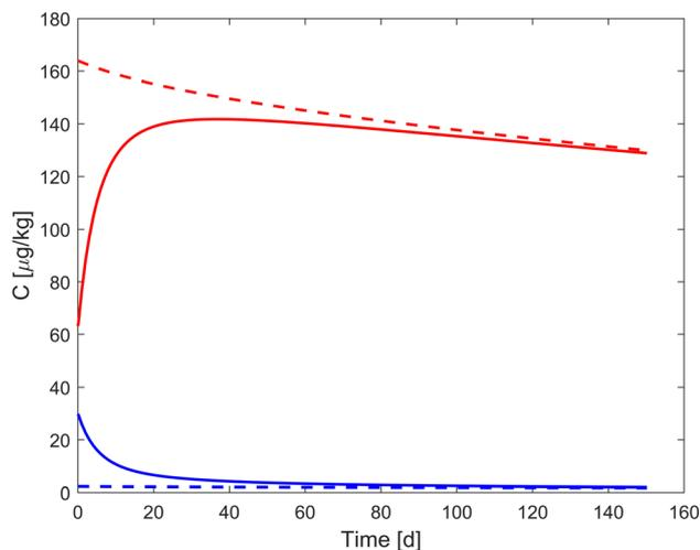
Fig. 2 Simulation of bezafibrate concentrations in the aqueous phase ( $C_w$ , blue) and averaged across all particle shells (red) in a non-sterile soil. Dashed lines indicate the equilibrium concentrations, based on the Freundlich-model, while solid lines indicate the simulation results with the calibrated model.
