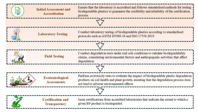
Fig. 6 Comprehensive laboratory-based certification protocol for biodegradable plastics.
