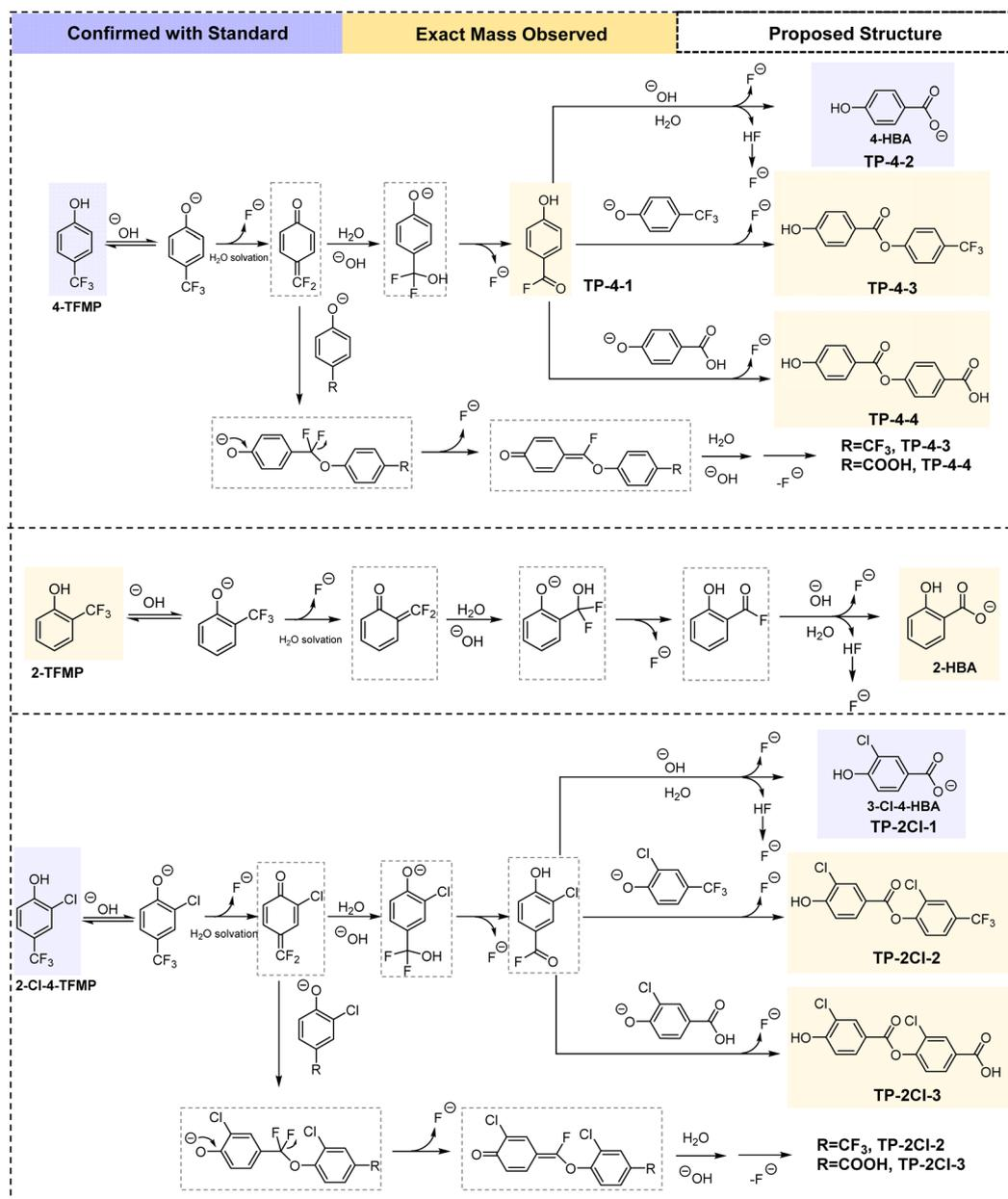
Fig. 3 Simplified proposed reaction mechanism for 4-TFMP, 2-TFMP, and 2-Cl-4-TFMP spontaneous aqueous defluorination. A detailed arrow-pushing mechanism can be found in Fig. S7.†
