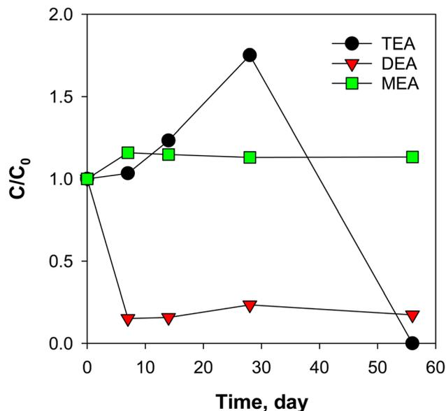
Fig. 5 Inoculation of Versalis E-cori corrosion inhibitor (1.7 mg mL<sup>-1</sup>) with PW2-Mar sample (2 mL) suggesting microbial transformations of ethanolamines. EDEA and MDEA were below the quantification limit of 1 µg L<sup>-1</sup>. Total volume = 60 mL, temperature = 21 °C.
