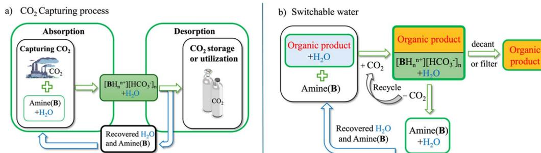
Fig. 1 Schematic illustration of using amines in the (a) CO<sub>2</sub> capture and (b) switchable water (SW) processes.
