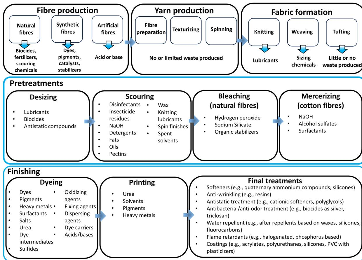
Fig. 2 Main processes involved in the textile supply chain and chemical category that can be released and discharged into wastewaters during each process. (Correia *et al.*,<sup>39</sup> 1994; Holkar *et al.*,<sup>40</sup> 2016; Khan *et al.*,<sup>14</sup> 2023; Lacasse and Baumann,<sup>2</sup> 2004).
