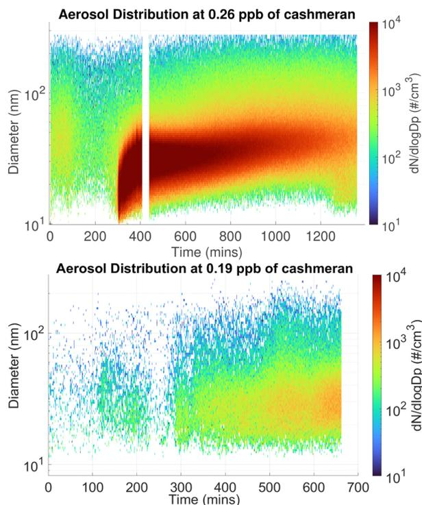
Fig. 7 Organic aerosol number concentration ( $dN/d \log D_p$ ) plot as a function of size and time from the SMPS for two experiments conducted under air at 292 K and 438 ppbv of excess  $O_3$ . The top and bottom graphs differ only in the concentration of cashmeran used.
