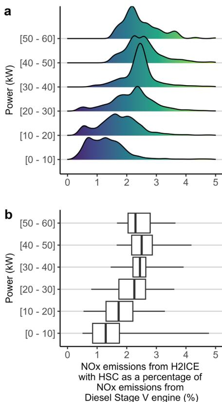
**Fig. 4** The difference in instantaneous  $\text{NO}_x$  emissions as a function of power setting between H2ICE with HSC and Stage V diesel engine for the across the NRTC. (a) Shows the distribution as density plots and (b) shows data as a box and whisker plot with median, interquartile and 5th and 95th percentile ranges.
