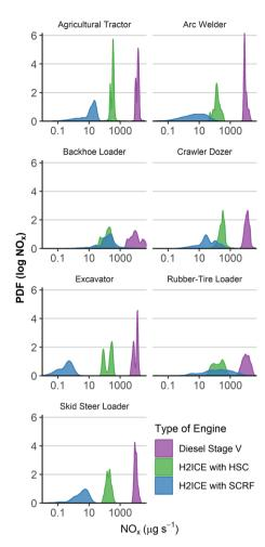
Fig. 5 NO<sub>x</sub> emissions distribution for the seven applications within the NRTC for (i) diesel Stage V, (ii) H2ICE with hydrogen slip catalyst (HSC), and (iii) H2ICE with selective catalytic reduction and particulate filter (SCRF).
