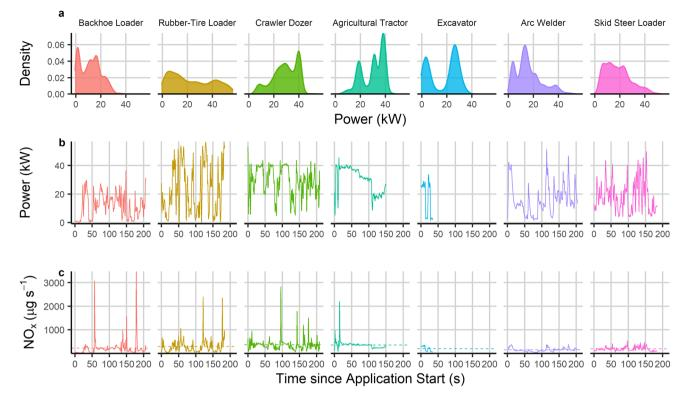
Fig. 6 H2ICE with hydrogen slip catalyst (HSC) for the hot-start non-road transient cycle. Showing (a) the density of the power, (b) the power (kW) during the application, and (c) the corresponding  $NO_x$  emissions where the dashed lines represent the mean value for each appliance.
