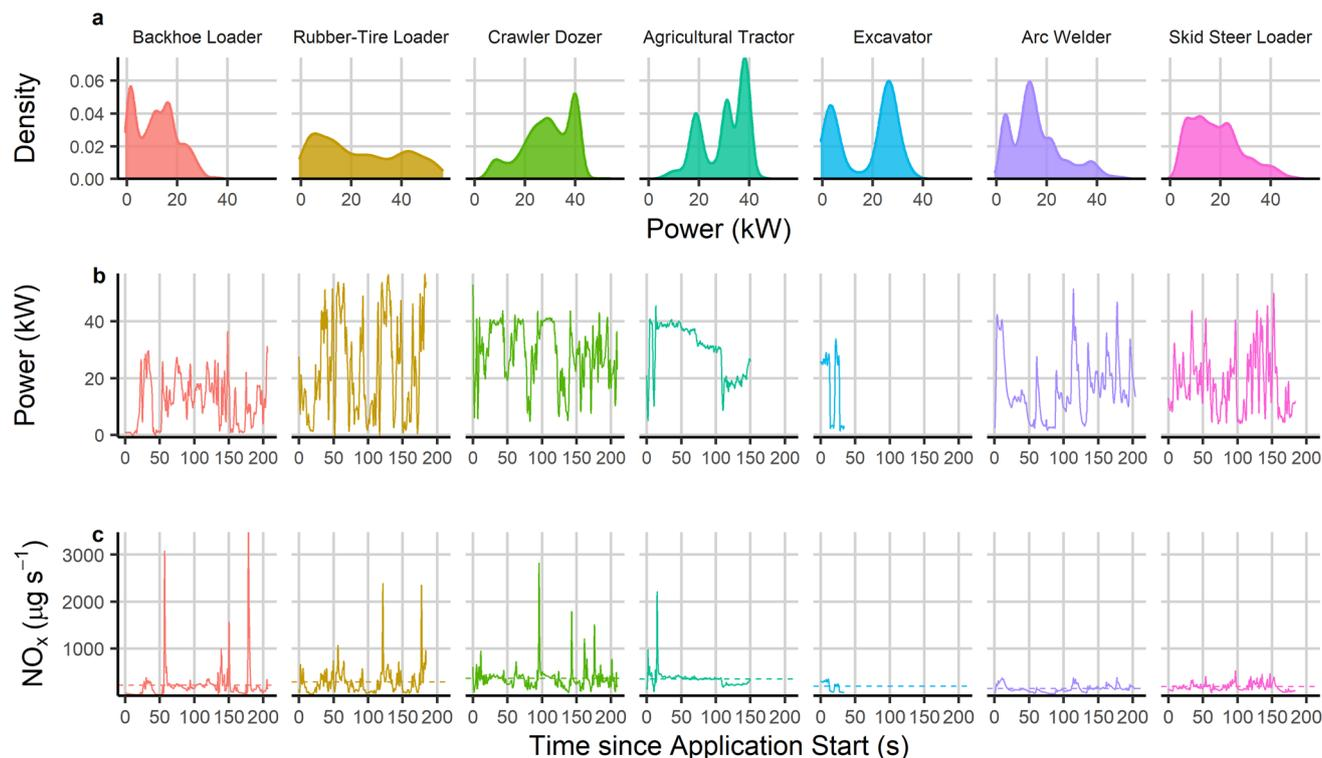
Fig. 6 H2ICE with hydrogen slip catalyst (HSC) for the hot-start non-road transient cycle. Showing (a) the density of the power, (b) the power (kW) during the application, and (c) the corresponding  $\text{NO}_x$  emissions where the dashed lines represent the mean value for each appliance.
