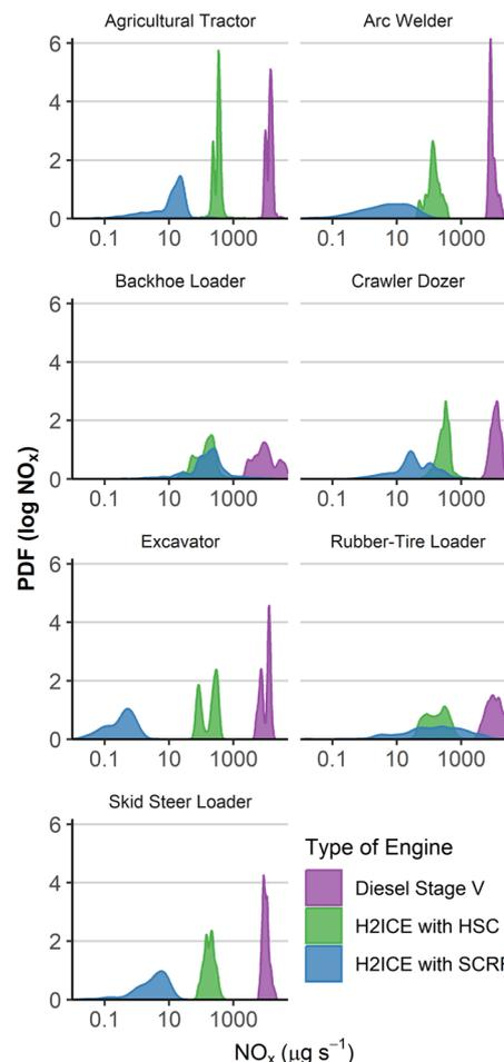
**Fig. 5**  $\text{NO}_x$  emissions distribution for the seven applications within the NRTC for (i) diesel Stage V, (ii) H2ICE with hydrogen slip catalyst (HSC), and (iii) H2ICE with selective catalytic reduction and particulate filter (SCRF).
