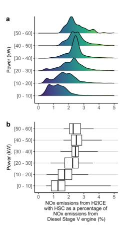
Fig. 4 The difference in instantaneous  $NO_x$  emissions as a function of power setting between H2ICE with HSC and Stage V diesel engine for the across the NRTC. (a) Shows the distribution as density plots and (b) shows data as a box and whisper plot with median, interquartile and 5th and 95th percentile ranges
