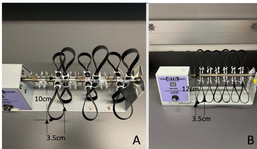
Fig. 1 Wristbands attached to two different types of end-over-end rotators: (A) small rotator set at 5 and 50 rpm (tangential velocities = 0.05 and 0.5  $\text{m s}^{-1}$ ). (B) Large rotator set at 85 rpm (tangential velocity = 1.1  $\text{m s}^{-1}$ ).
