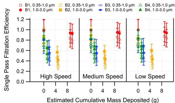
Fig. 4 SPFE results for CR boxes as a function of cumulative mass deposited at 0, 30, and 40 weeks. Error bars represent an estimate 20% relative error on the SPFE measurement.
