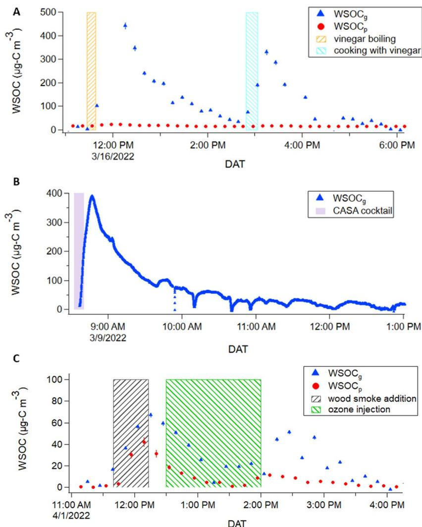
Fig. 4 Indoor  $WSOC_g$  (blue triangles) and  $WSOC_p$  concentrations (red dots) in indoor air during selected perturbations.
