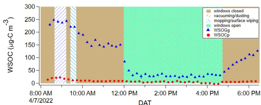
Fig. 3 Indoor  $WSOC_g$  (blue triangles) and  $WSOC_p$  concentrations (red dots) during surface cleaning of the wood smoke contaminated house (cleaning times indicated by purple and blue-bands), window opening (green band) and subsequent window closing (brown band). Error bars represent measurement uncertainties ( $\pm 1 \sigma$ ) and are mostly smaller than the data point markers (DAT = date and time).
