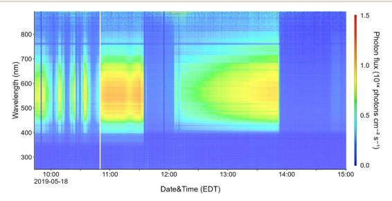
Fig. 3 Time series of photon flux taken inside the Toyota on May 18, 2019. Data was not available for a short period at 10:50 a.m.; this is reflected by the white pixels at all wavelengths at that time.
