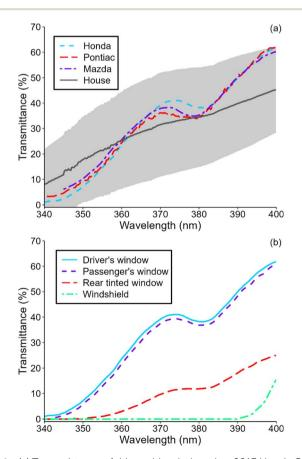
Fig. 2 (a) Transmittance of driver-side windows in a 2013 Honda CRV, a 2006 Pontiac G6 sedan, and a 2016 Mazda 3 hatchback. Average transmittance of 13 windows in 13 single-family residences (standard deviation in shaded grey) is also shown for reference.23 (b) Transmittance of various windows in the Honda CRV.
