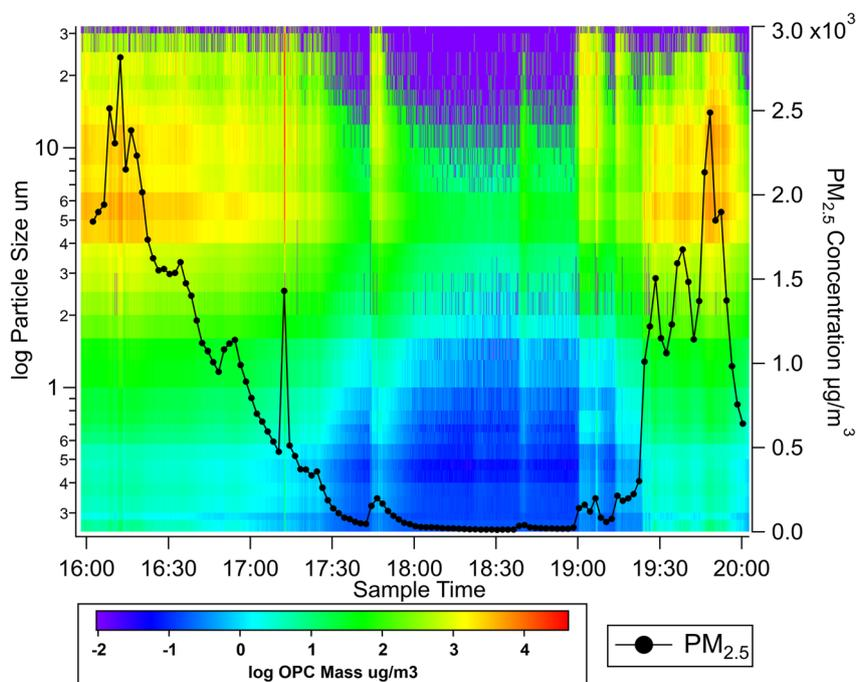
Fig. 5 2-D plot of the mass concentration distribution of all particle sizes throughout the experimental period. Temporal profile of  $\text{PM}_{2.5}$  concentration is illustrated against the right axis.
