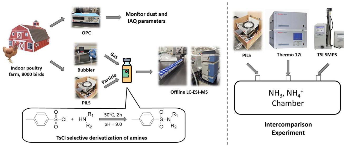
Fig. 1 Layout of sample collection, derivatization, analysis, and inter-comparison. OPC: optical particle counter, IAQ: indoor air quality, PILS: particle into liquid sampler, TsCl: *p*-toluenesulfonyl chloride, LC-ESI-MS: liquid chromatography electrospray ionization mass spectrometry, SMPS: scanning mobility particle sizer.
