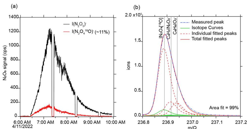
Fig. 7 (a) Adding labeled  $O_3$  to the house enhanced  $^{18}O$ - $N_2O_5$ . (b) The I-CIMS separates  $^{18}O$ -substituted  $N_2O_5$  from adjacent ion peaks in the mass spectrum. Note that the timeseries includes periodic zero air measurements; signals decrease during this time.
