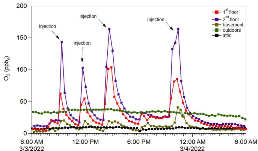
Fig. 6 Ozone concentrations (ppb) on 3 March 2022 as detected from inlet lines located on the 1st (red), 2nd (purple), and basement (brown) floors in contrast to the outdoor (green) concentrations.
