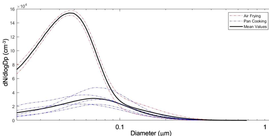
Fig. 11 Average particle size distributions sampled in the dining room during all air frying and pan cooking events. Each dashed curve represents one average size distribution for one cooking event (air frying in red and pan frying in blue). Averages for air frying and pan cooking are represented by the dark lines.
