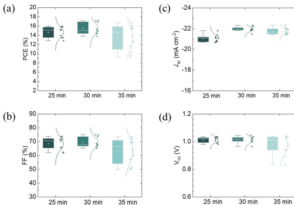
Fig. 3 Performance statistics extracted from the  $JV$  curves obtained under simulated solar illumination for devices that have been converted using the 25 min, 30 min and 35 min processes. (a) PCE (b) FF (c)  $J_{sc}$ , and (d)  $V_{oc}$ .
