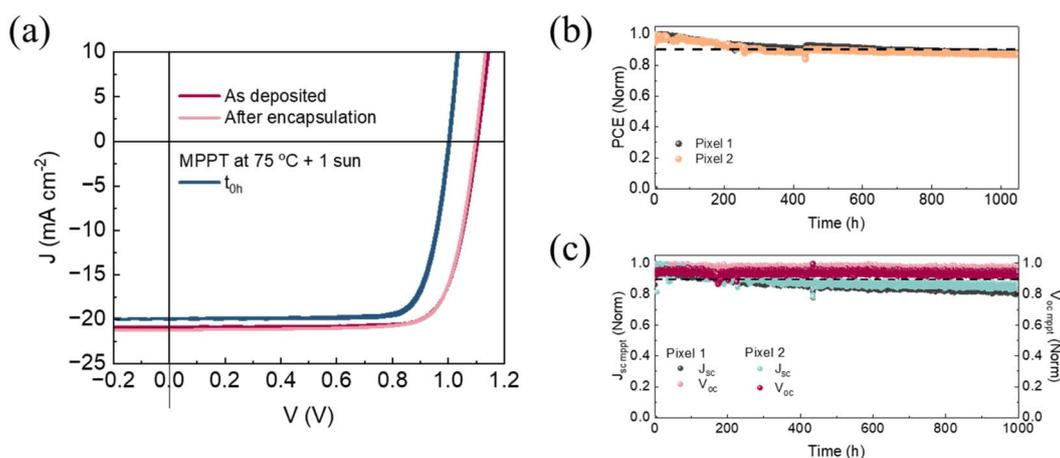
Fig. 6 (a) *JV* curves measured at different stages: as-deposited, after encapsulation, and after mpp tracking testing at 75 °C under 1 sun illumination at  $t_0$ . (b) Normalized power output of the device during mpp tracking operation of two different pixels. (c) Normalized evolution of  $J_{sc}$  and  $V_{oc}$  during mpp tracking of two different pixels.
