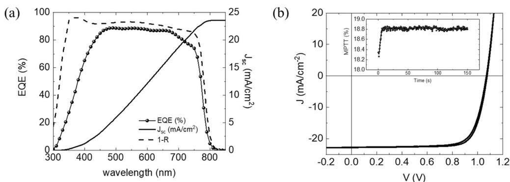
Fig. 4 (a) External quantum efficiency and 1-reflectance curves. (b)  $JV$  curve for the best pixel with stabilized power output measured for 100 s in the inset.
