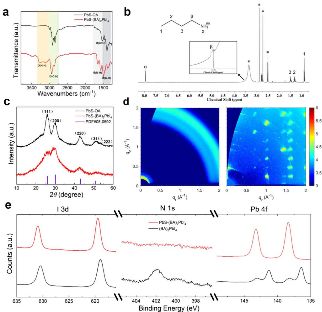
Fig. 3 (a) FTIR spectra of PbS CQDs before and after ligand-exchange. (b) <sup>1</sup>H NMR spectrum of PbS-(BA)<sub>2</sub>PbI<sub>4</sub>. (c) XRD patterns of PbS-OA and PbS-(BA)<sub>2</sub>PbI<sub>4</sub> films. (d) GIWAXS patterns of neat (BA)<sub>2</sub>PbI<sub>4</sub> and PbS-(BA)<sub>2</sub>PbI<sub>4</sub> CQDs thin films. (e) XPS profiles of (BA)<sub>2</sub>PbI<sub>4</sub> (black line) and PbS-(BA)<sub>2</sub>PbI<sub>4</sub> (red line) films, showing I 3d, Pb 4f, and N 1s bands.
