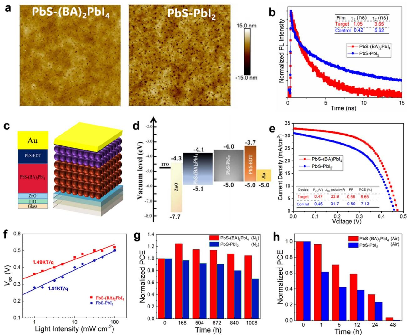
Fig. 5 Comparison of  $\text{PbS}-(\text{BA})_2\text{PbI}_4$  and  $\text{PbS-PbI}_2$  CQD films and devices. (a) TP-AFM images and (b) TRPL spectra. (c) Schematic of CQD solar cells with (d) energy band structures, and (e)  $J-V$  curves. (f) Light intensity dependences of  $V_{oc}$  for CQD devices. Lifetime curves of CQD devices after storage in (g) Ar and (h) air (80–90% RH) atmospheres.
