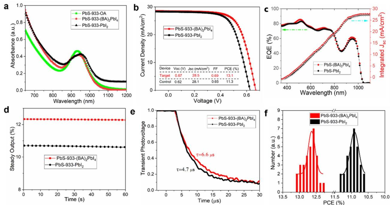
Fig. 6 (a) UV-Vis-IR light absorption spectra of PbS-933-OA in solution and PbS-933-(BA)<sub>2</sub>PbI<sub>4</sub> and PbS-933-PbI<sub>2</sub> in thin films. (b)  $J$ - $V$  curves, (c) EQE spectra, (d) steady output of PCEs at maximum power points over 60 s, (e) transient photovoltage, and (f) PCE distribution of solar cells based on PbS-933-(BA)<sub>2</sub>PbI<sub>4</sub> and PbS-933-PbI<sub>2</sub> films.
