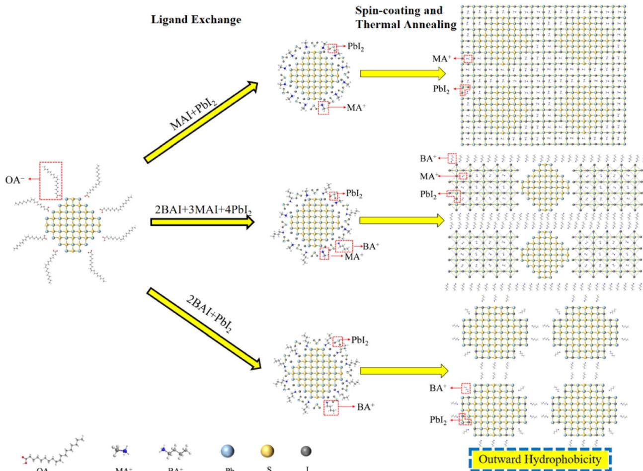
Fig. 4 Illustration of film-forming processes of  $\text{PbS-MAPbI}_3$ ,  $\text{PbS}-(\text{BA})_2(\text{MA})_4\text{Pb}_5\text{I}_{16}$ , and  $\text{PbS}-(\text{BA})_2\text{PbI}_4$  via a sequence of ligand-exchange and spin-coating followed by thermal annealing.
