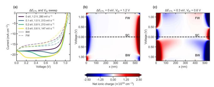
Fig. 9 (a) Simulated transient J-V curves for various energetic level configurations, showing the same  $J_{SC}$  loss due to ionic screening, which occur at slightly different scan rates as the energetic alignment also influences the J-V hysteresis timescales.  $\Delta E_{CTL}$  and  $V_{bj}$  are varied in parallel. Ionic charge profiles during the J-V scans in (a) for (b) perfectly aligned contacts with high  $V_{\rm bi}$  and (c) large energetic offset with low  $V_{\rm bi}$
