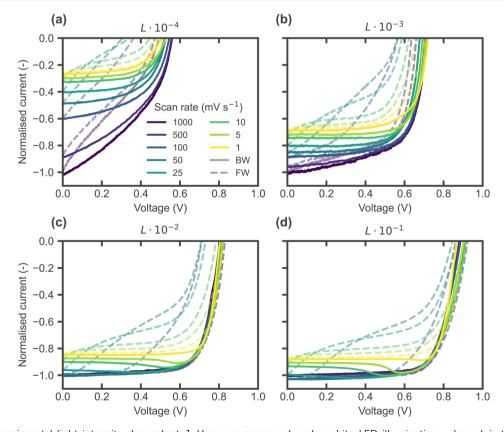
Fig. 10 (a)–(d) Experimental light intensity-dependent J-V curves measured under white LED illumination, where L is the maximum light intensity of the LED, equivalent to  $\approx$  1.5 sun intensity. The J-V curves were measured starting with the backward scan from a precondition at  $V_{\rm OC}$ for each scan rate. The  $J_{SC}$  level difference across scan rates increases with decreasing light intensity due to slow capacitive effects becoming more prominent at low intensities.
