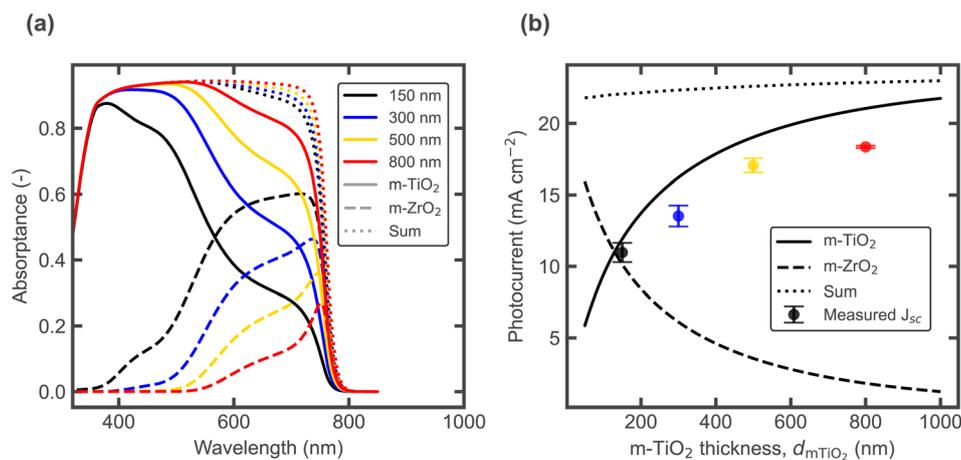
Fig. 3 (a) Simulated layer absorbance for varying  $m\text{-TiO}_2$  thickness, with a constant 1000 nm  $m\text{-ZrO}_2$  layer, using an effective medium approximation with 65% MAPbI<sub>3</sub> and 35% oxide. (b) Simulated 1 sun photocurrent (sum) and contribution from each layer, plotted together with the experimental steady state  $J_{sc}$  values from Fig. 2b.
