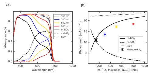
Fig. 3 (a) Simulated layer absorptance for varying m-TiO $_2$  thickness, with a constant 1000 nm m-ZrO $_2$  layer, using an effective medium approximation with 65% MAPbI $_3$  and 35% oxide. (b) Simulated 1 sun photocurrent (sum) and contribution from each layer, plotted together with the experimental steady state  $J_{SC}$  values from Fig. 2b.
