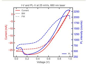
Fig. 8 Experimental I-V and PL-V curves under illumination with a red (660 nm) laser. Axes of I and PL have been arbitrarily aligned.
