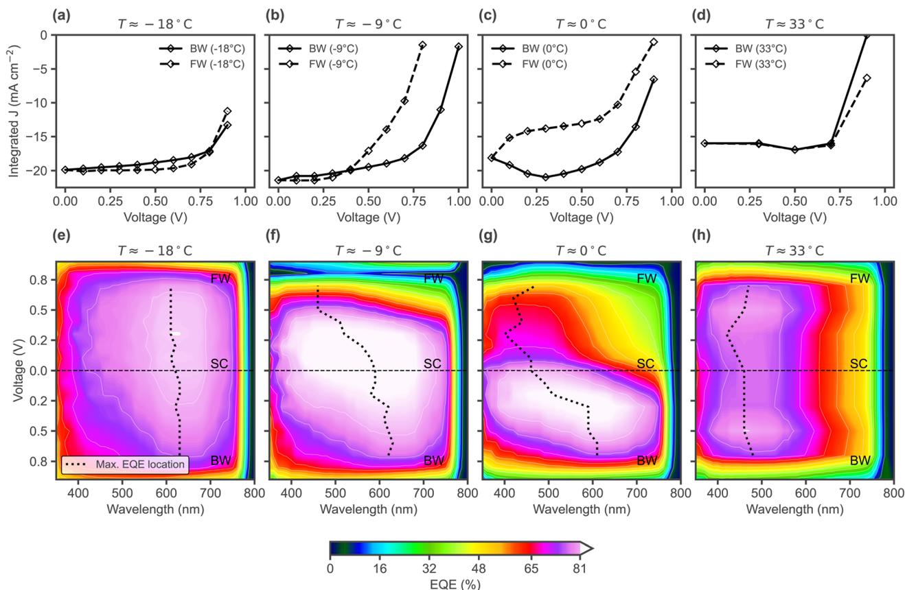
Fig. 7 (a)–(d) Experimental  $J$ - $V$  curves reconstructed from the EQE( $V$ ) spectra (using 1 sun AM 1.5G spectrum for the integration), measured under different temperatures, starting with the BW scan from a precondition at 1 V. (e)–(h) Contour maps of EQE- $V$  profiles for different device temperatures, showing the wavelength location of the maximum EQE at each bias voltage.
