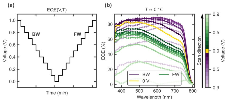
**Fig. 6** (a) Measurement procedure, recording EQE spectra at each bias voltage level in a staircase order, where each EQE measurement takes  $\approx 2$ -3 min. (b) Experimental EQE spectra measured under different bias voltages in order, starting with the BW scan from a forward bias precondition (cooling to  $0^\circ\text{C}$  under 1 V).
