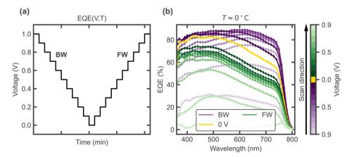
Fig. 6 (a) Measurement procedure, recording EQE spectra at each bias voltage level in a staircase order, where each EQE measurement takes  $\approx 2-3$  min. (b) Experimental EQE spectra measured under different bias voltages in order, starting with the BW scan from a forward bias precondition (cooling to 0 °C under 1 V).
