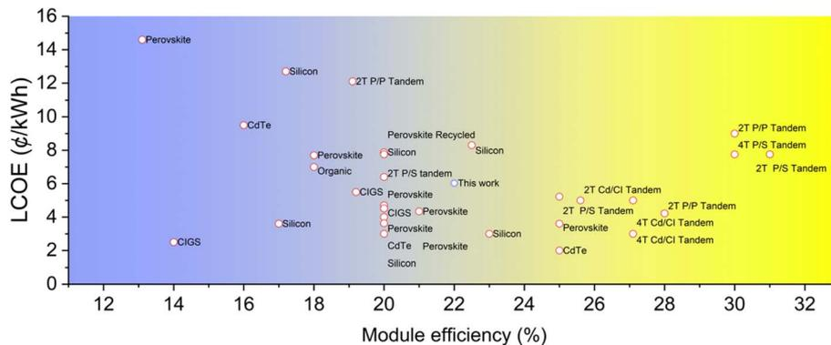
Fig. 7 LCOE vs. module efficiency comparison across various PV technologies published in the literature, with LCOE data collected from ref. 84–104.
