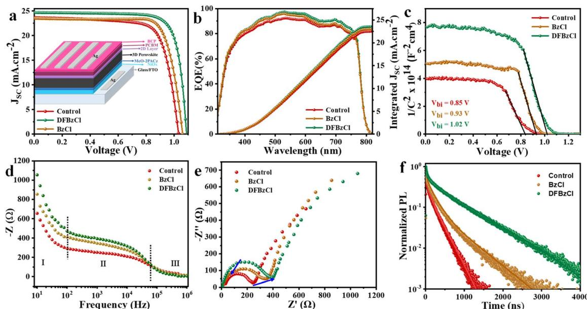
Fig. 3 (a) *J*–*V* characteristics of the control device and modified with BzCl and DFBzCl devices (inset: device architecture). (b) External quantum efficiency (EQE) and integrated current density as a function of wavelength for all three devices. (c) Mott–Schottky curve, (d) Bode plot with frequency (e) Nyquist plot for control, BzCl and DFBzCl devices under illumination. (f) Time-resolved PL curve for all three films measured by time-correlated single photon counting (TCSPC) measurement.
