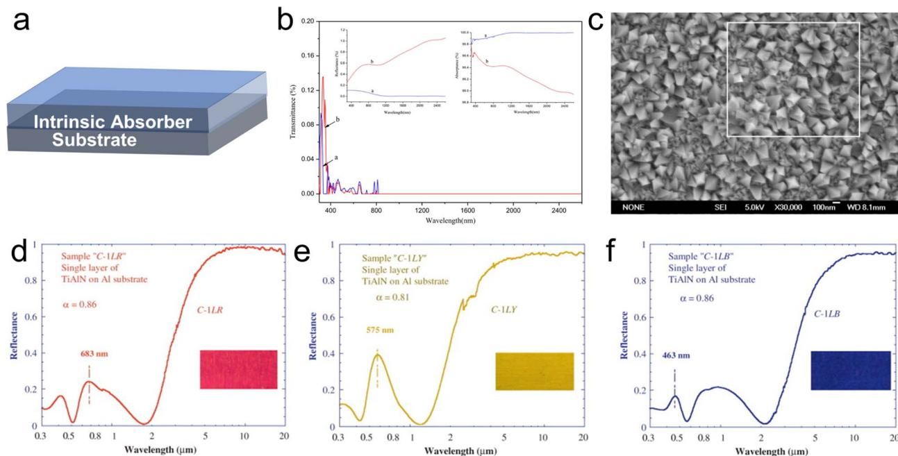
Fig. 6 Fundamentals and recent advances in intrinsic SSACs. (a) Structural schematic of intrinsic SSACs. (b) Transmittance, reflectance, and absorbance spectra and (c) SEM image of CrAlN films.<sup>96</sup> Copyright 2014, Elsevier. (d–f) Reflectance spectra of TiAlN SSACs with various colors.<sup>69</sup> Copyright 2010, Elsevier.
