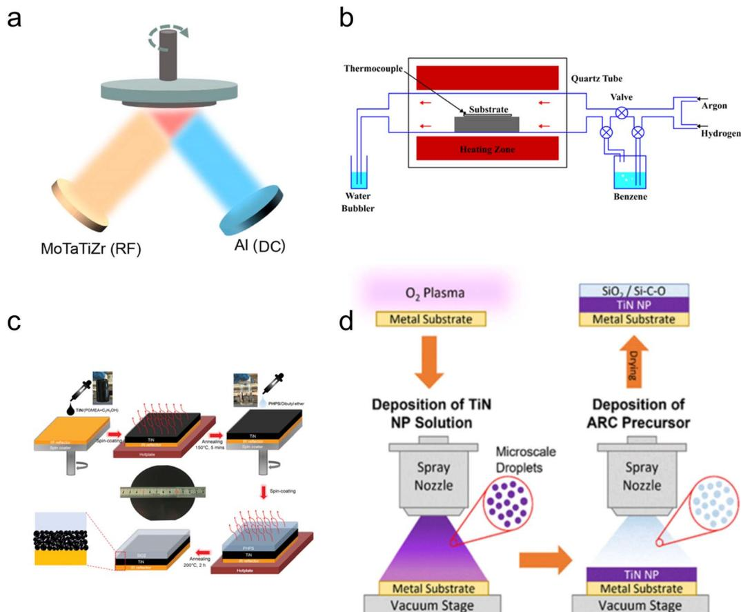
Fig. 5 Fabrication method for SSACs. Schematic illustrations of (a) magnetron sputtering,<sup>21</sup> Copyright 2022, Elsevier. (b) CVD,<sup>54</sup> Copyright 2014, Wiley-VCH; (c) spin coating,<sup>56</sup> Copyright 2020, Wiley-VCH and (d) spray coating.<sup>57</sup> Copyright 2025, Engineered Science.
