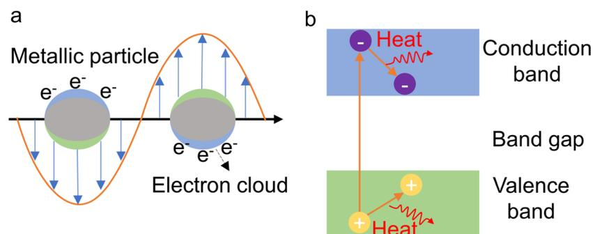
Fig. 2 Schematic illustration of (a) the localized surface plasmon resonance effect and (b) absorption *via* interband electronic transitions.
