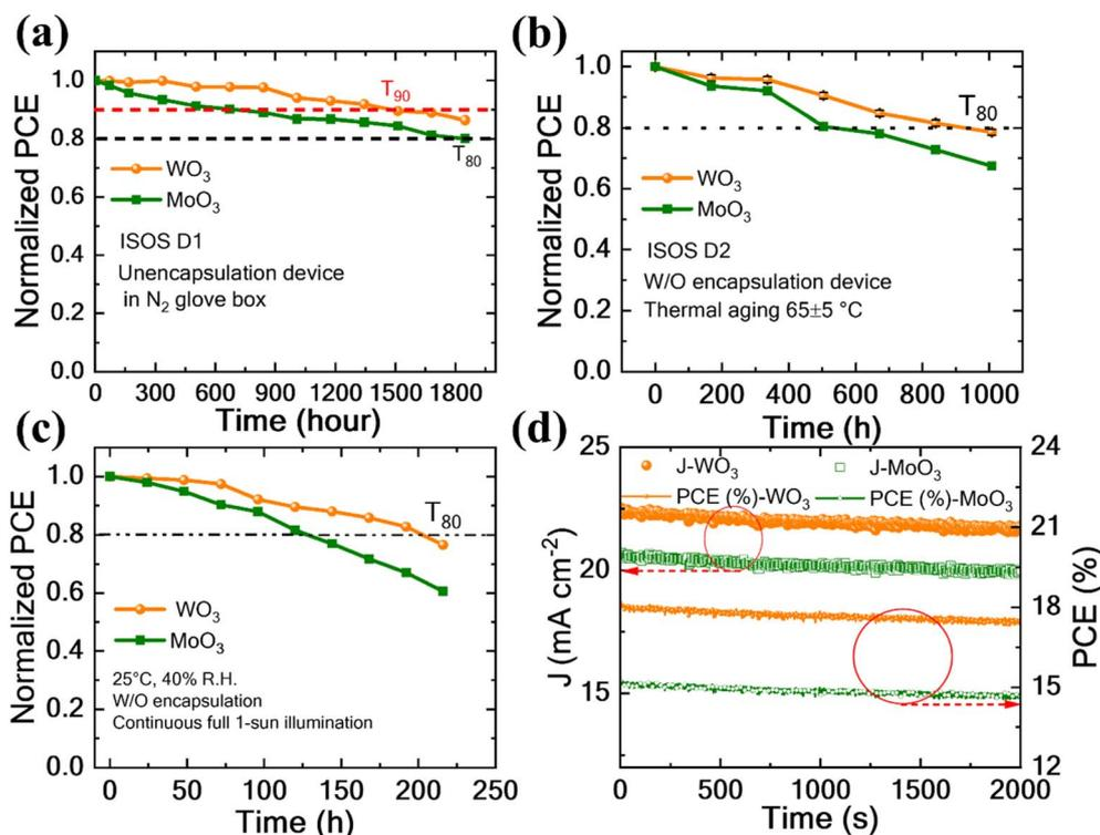
Fig. 5 Stability analysis of the d-block MO-based T-PSCs. (a) Shelf-life stability inside an  $N_2$ -filled glove box, (b) thermal stability test at continuous  $65 \pm 5 \text{ }^\circ\text{C}$  placed inside a muffle furnace, (c) light stability test under continuous 1-sun illumination (with an LED lamp), and (d) steady state PCE tracking at a constant voltage under 1-sun illumination of the unencapsulated T-PSCs.
