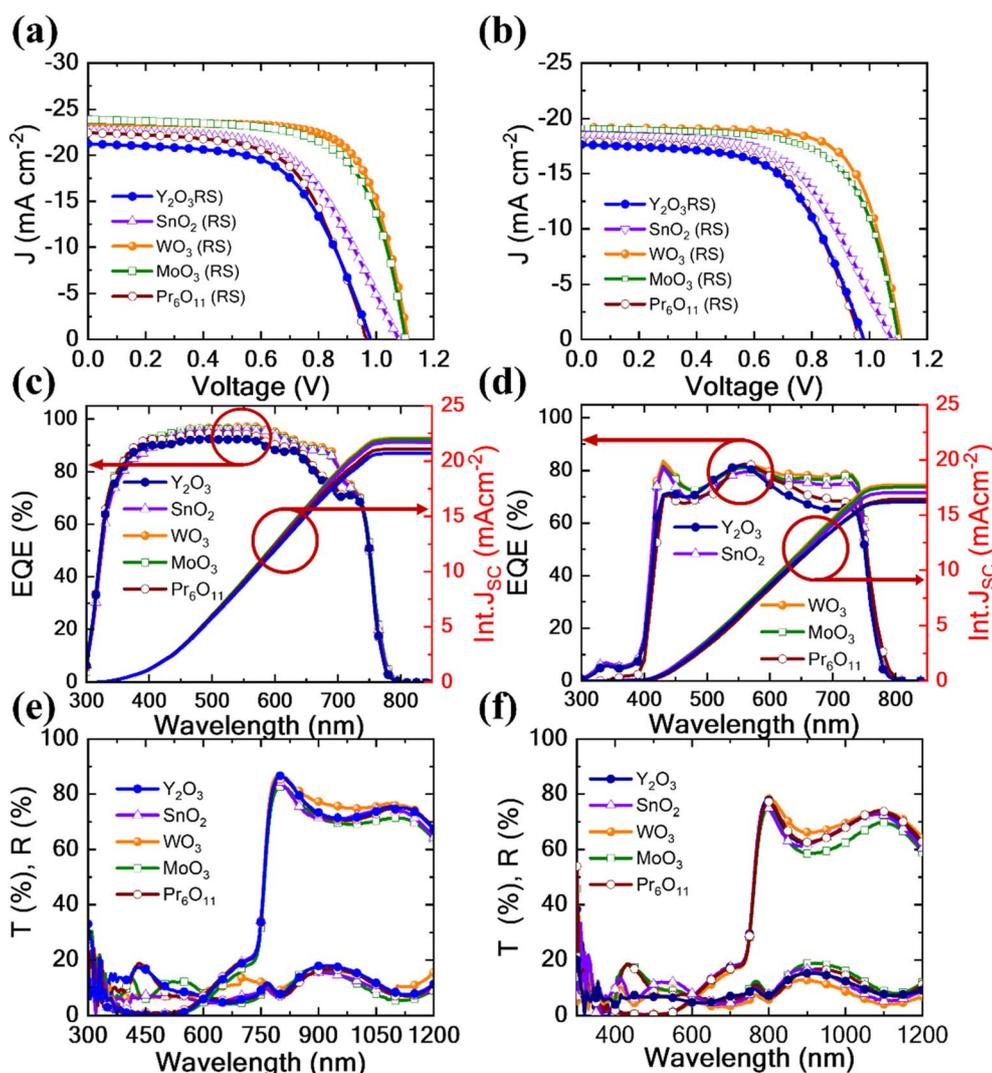
Fig. 4 Photovoltaic properties of the varying MO incorporating T-PSCs. (a) and (b).  $J-V$  characteristics under 1-sun conditions (AM 1.5 G;  $100 \text{ mW cm}^{-2}$ ) (c) and (d) EQE with  $\text{Int. } J_{SC}$  and (e) and (f) transmission spectra of the T-PSCs under (a, c, and e) bottom and (b, d, and f) top side illumination conditions.
