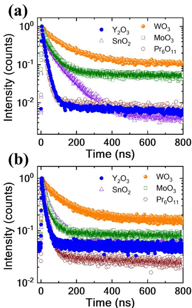
Fig. 3 Carrier lifetime analysis of the perovskite thin films with varying MO incorporation. TCSPC decay spectra of the perovskite thin films having different MO layers under (a) bottom and (b) top side illumination conditions.
