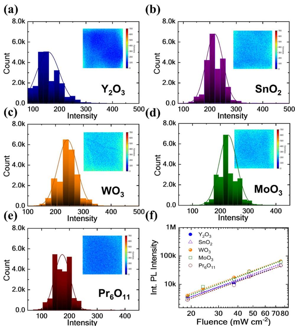
Fig. 2 Radiative intensity of the perovskite thin films with varying MO incorporations. (a)–(e) PL intensity distribution over a pixel area of  $160 \times 190$  with different MO-based perovskite thin films, (inset: a PL image of the corresponding sample), and (f) linear fitting of the fluence-dependent PL analysis.
