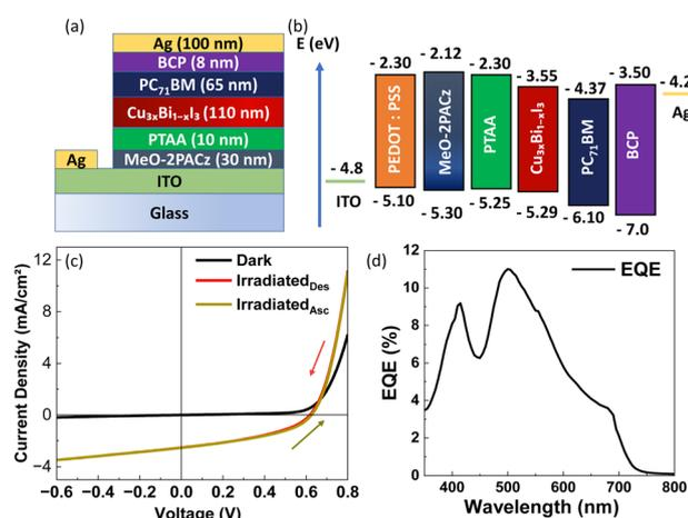
**Fig. 4** (a) Architecture of the  $\text{Cu}_{3x}\text{Bi}_{1-x}\text{I}_3$  solar cells. (b) Relevant charge carrier transport energies of the individual layers from the architecture (and also of PEDOT:PSS). (c)  $J-V$  curve of the champion solar cell in the dark and under illumination, measured in forward and reverse directions. (d) The External Quantum Efficiency (EQE) shows photocurrent generation up to 740 nm matching the optical band gap of  $\text{Cu}_{3x}\text{Bi}_{1-x}\text{I}_3$ .
