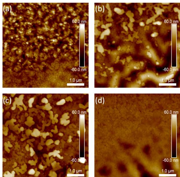
**Fig. 3** Atomic Force Micrographs show the topography of  $\text{Cu}_{3x}\text{Bi}_{1-x}\text{I}_3$  deposited on (a) PEDOT:PSS, (b) MeO-2PACz, (c) PTAA and (d) PTAA on top of MeO-2PACz. The overall film homogeneity is satisfactory atop PEDOT:PSS and rather poor atop either MeO-2PACz or PTAA due to wetting issues. The film roughness and resulting device performance was maximized using a bilayer of PTAA and MeO-2PACz (d).
