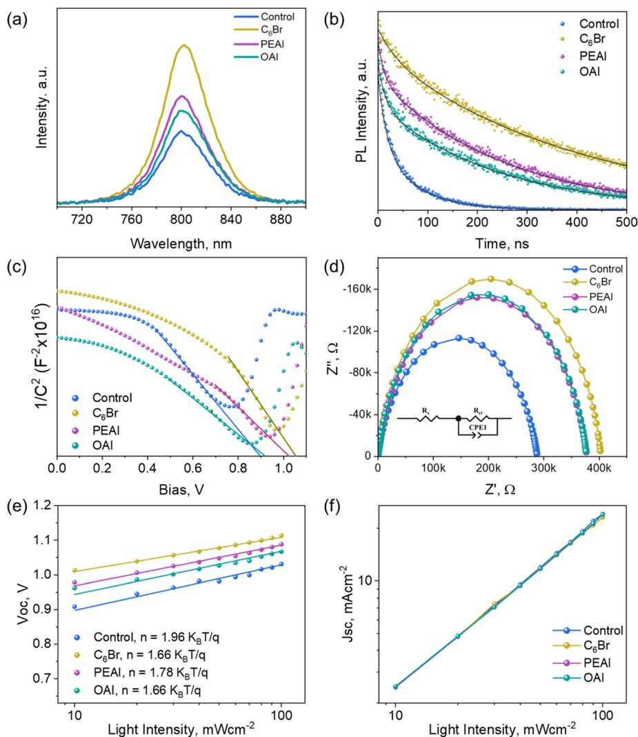
Fig. 4 (a) Steady-state photoluminescence (PL) spectra, (b) time-resolved photoluminescence (TRPL) decay curves, (c) capacitance–voltage ( $C$ – $V$ ) profiles, (d) electrochemical impedance spectroscopy (EIS) Nyquist plots, (e) dependence of open-circuit voltage ( $V_{oc}$ ) on illumination intensity, and (f) dependence of short-circuit current density ( $J_{sc}$ ) on illumination intensity for devices employing various 2D passivation layers.
