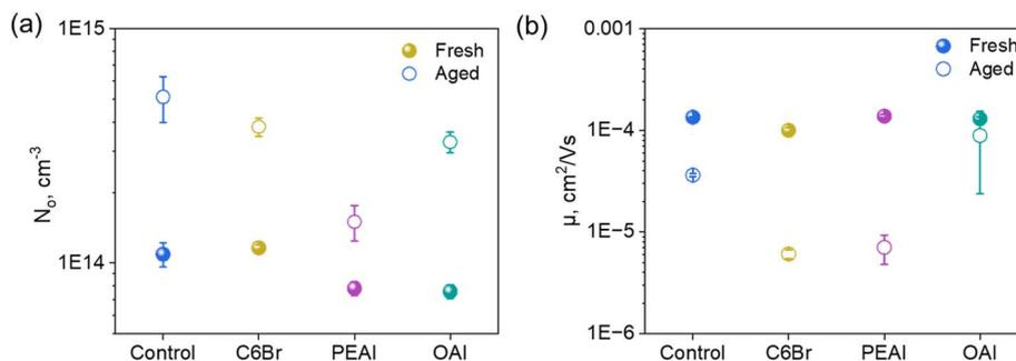
Fig. 6 (a) Mobile ion concentration ( $N_0$ ), and (b) ionic mobility ( $\mu$ ) measured in fresh and aged perovskite solar cell devices with different 2D passivation layers: control, C<sub>6</sub>Br, PEAI, and OAI. Fresh devices are represented by solid dots and aged devices by circles.
