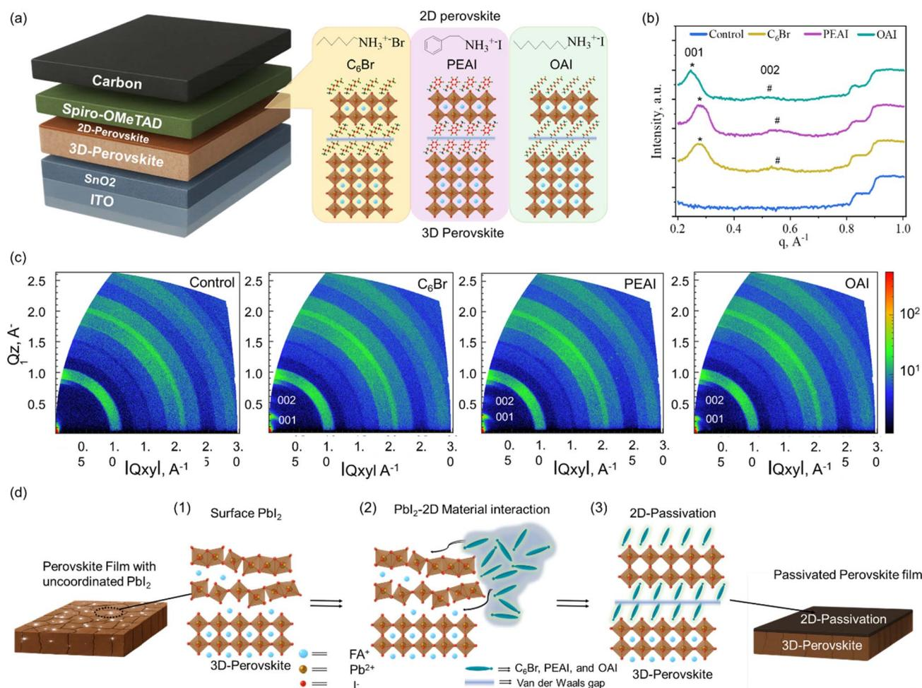
**Fig. 1** (a) Schematic of the perovskite solar cell architecture with 2D passivation layers (C<sub>6</sub>Br, PEAI, and OAI, respectively); (b) normalized in-plane GIWAXS intensity profiles; (c) 2D GIWAXS patterns showing 001/002 Ruddlesden–Popper-phase reflections indicating 2D perovskite formation; (d) illustration of the 2D passivation mechanism involving surface PbI<sub>2</sub> interaction, 2D layer formation, and passivated interface development.
