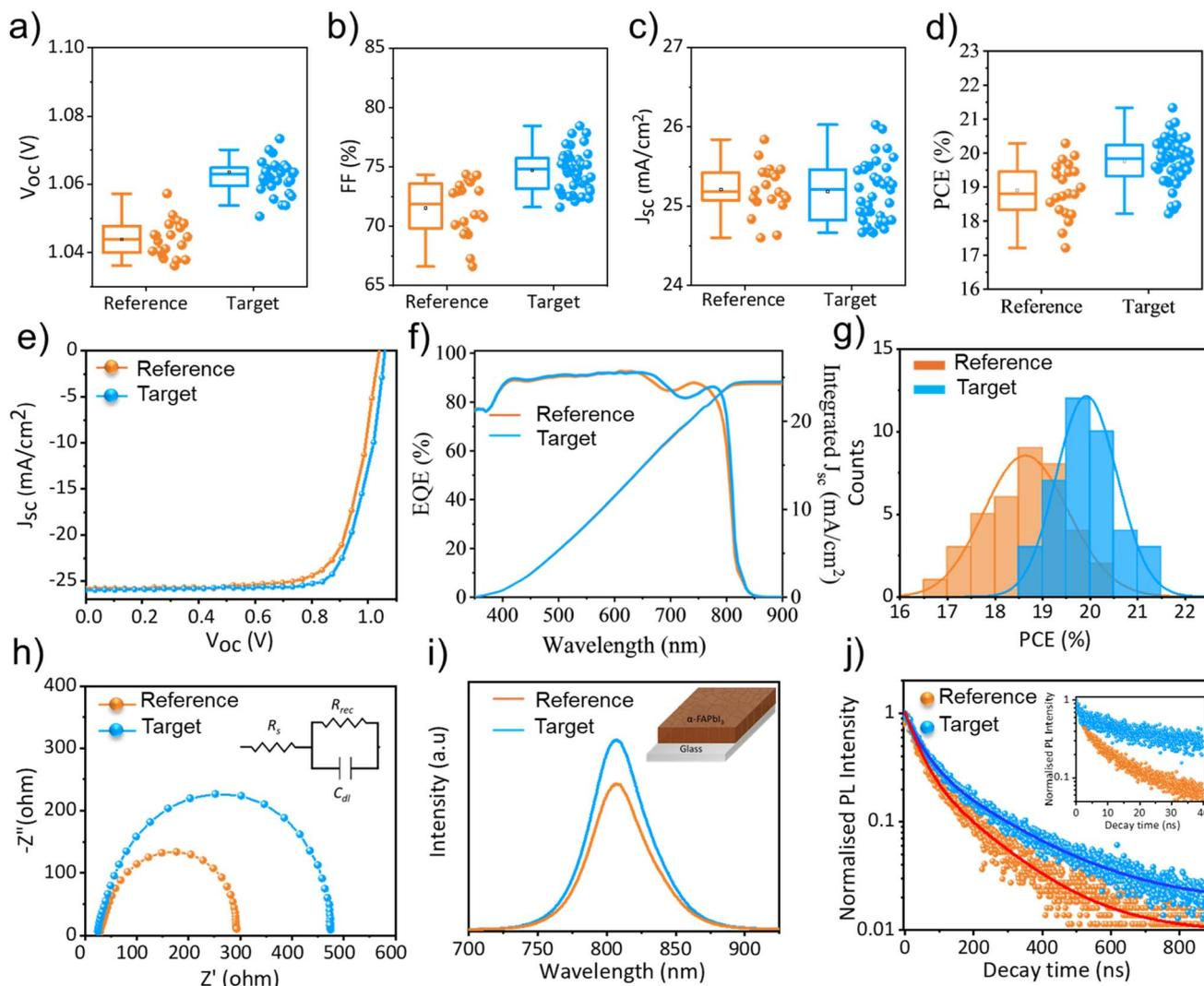
Fig. 4 Statistical distribution of the PV parameters (a)  $V_{oc}$ , (b) FF, (c)  $J_{sc}$  and (d) PCE of reference and target (oxygen-induced) perovskite-based solar cells. (e)  $J$ - $V$  characteristics and (f) EQE spectra of the best-performing devices. (g) PCE of 30 devices for each device type of the reference and target PSCs. (h) EIS Nyquist plots of the best-performing reference and target devices. (i) PL spectra and (j) TRPL decays of perovskite films.
