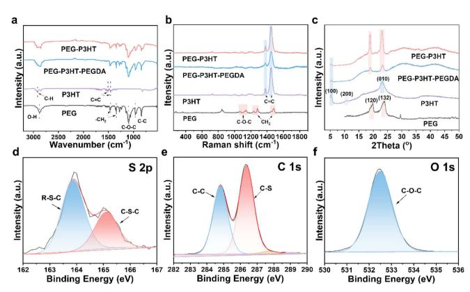
Fig. 2 Molecular characterization of PEG-P3HT hydrogels. (a–c) FTIR, Raman, and XRD spectra demonstrating successful incorporation of P3HT into the PEG-4SH network. (d–f) S 2p, C 1s, and O 1s XPS spectra of PEG-P3HT hydrogel.
