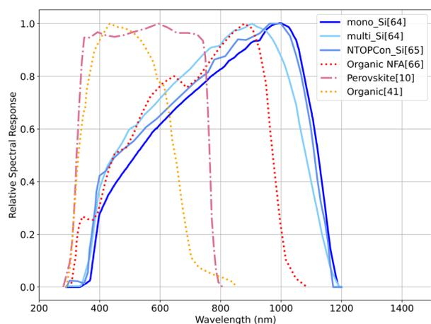
Fig. 4 Normalised spectral responses of different PVs.<sup>10,41,64–66</sup>
