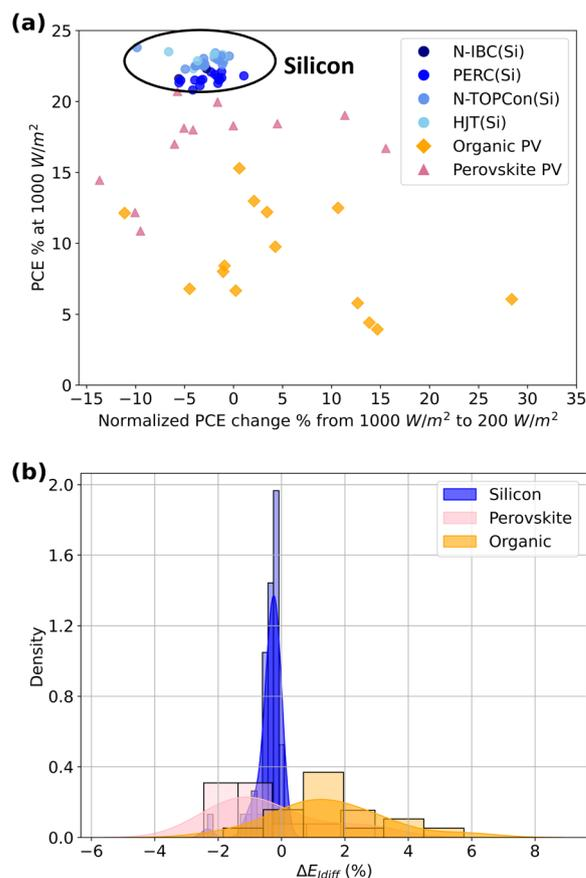
Fig. 3 (a) Difference in PCE measured at  $1000$  and  $200 \text{ W m}^{-2}$  for different reported PV technologies and (b) histogram (bars) with accompanying kernel density estimation (curves) of  $E_{\text{Idiff}}$  predicted for California City (2019) for populations of PVs in the dataset.
