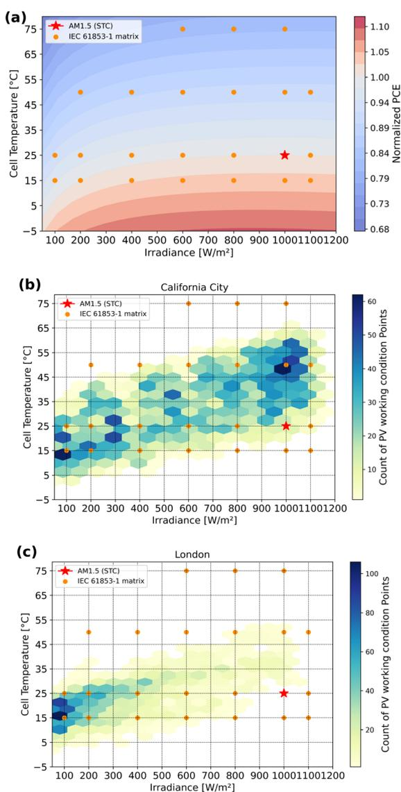
Fig. 1 (a) Normalised PCE of commercial silicon PVs<sup>2</sup> under different irradiance and temperature conditions, (b) density of real operation conditions of silicon PVs in California 2019 and (c) London 2019.
