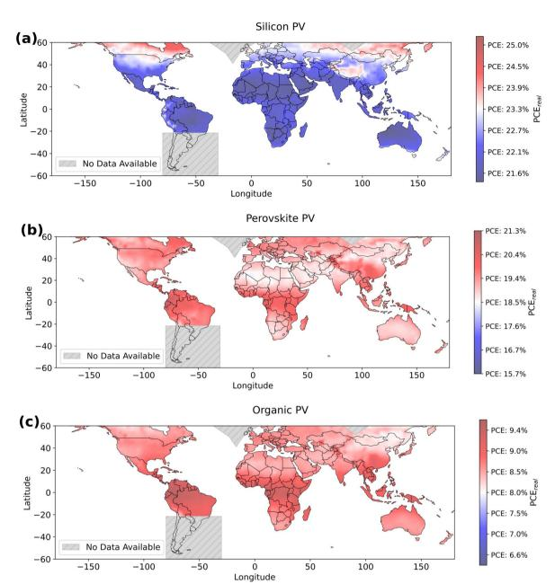
Fig. 6 (a) Predicted PCE<sub>real</sub> compared to PCE<sub>STC</sub> for silicon PVs across the world in 2019, (b) the corresponding map for perovskite PVs and (c) for organic PVs.
