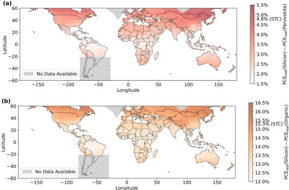
Fig. 7 The comparison of PCE<sub>real</sub> gap across the world in 2019 between silicon and (a) perovskite PVs and (b) organic PVs.
