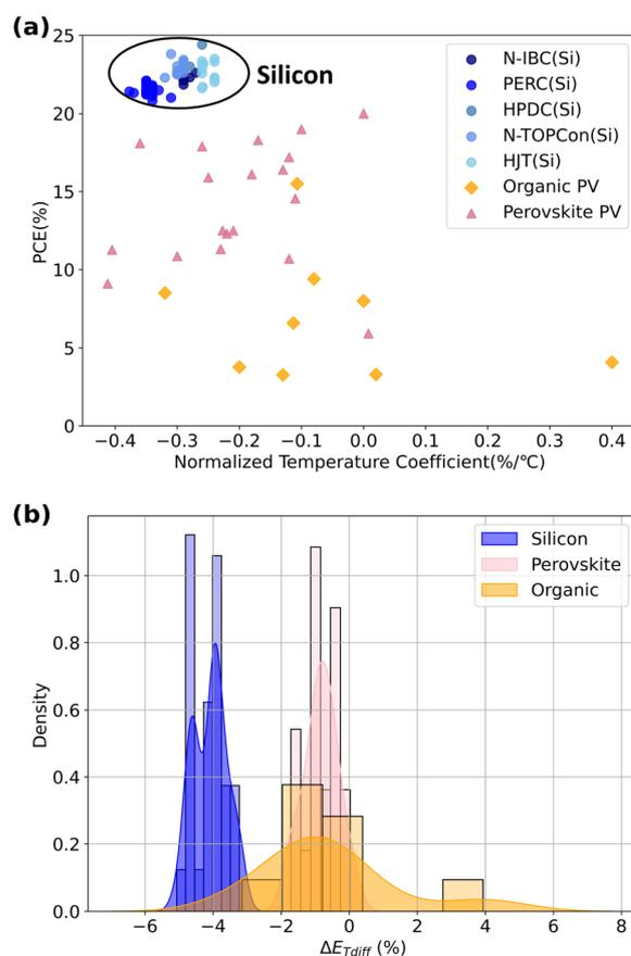
Fig. 2 (a) Temperature coefficient and PCE measured at  $25 \text{ }^\circ\text{C}$  for different reported PV technologies and (b) histogram (bars) with accompanying kernel density estimation (curves) of  $E_{T\text{diff}}$  predicted for California City (2019) for populations of PVs in the dataset.
