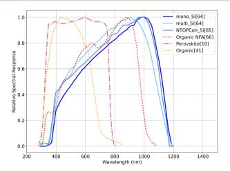
Fig. 4 Normalised spectral responses of different PVs. 10,41,64-66
