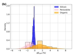
Fig. 3 (a) Difference in PCE measured at 1000 and 200 W m<sup>-2</sup> for different reported PV technologies and (b) histogram (bars) with accompanying kernel density estimation (curves) of  $E_{\text{Idiff}}$  predicted for California City (2019) for populations of PVs in the dataset.
