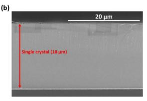
Fig. 3 SEM cross-section of a single-crystalline MAPbCl<sub>3</sub> thin film solar cell (a) with a thickness of  $\sim$ 4  $\mu$ m (b) with a thickness of  $\sim$ 18  $\mu$ m.
