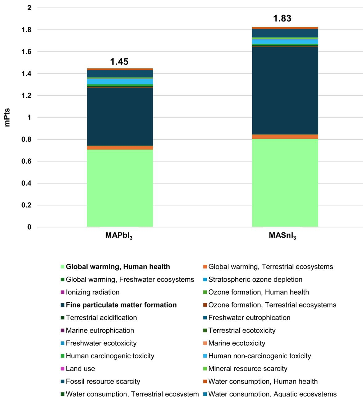
Fig. 3 Endpoint single score characterization for the synthesis of 1 g of MAPbI<sub>3</sub> and MASnI<sub>3</sub> 40 wt% in DMF.
