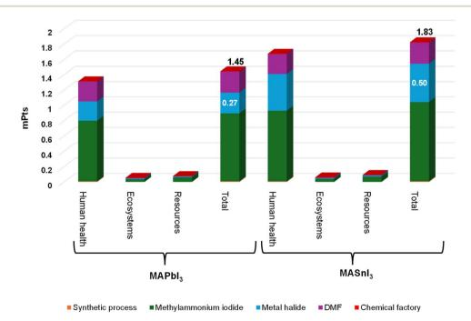
Fig. 4 Endpoint single score (mPts) characterization for the synthesis of 1 g of MAPbl<sub>3</sub> and MASnl<sub>3</sub> (40 wt% in DMF). Focus of the component contribution into the three damage areas.
