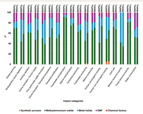
Fig. 2 Midpoint characterization for the synthesis of 1 g of MAPbl<sub>3</sub> and MASnl<sub>3</sub> 40 wt% in DMF.
