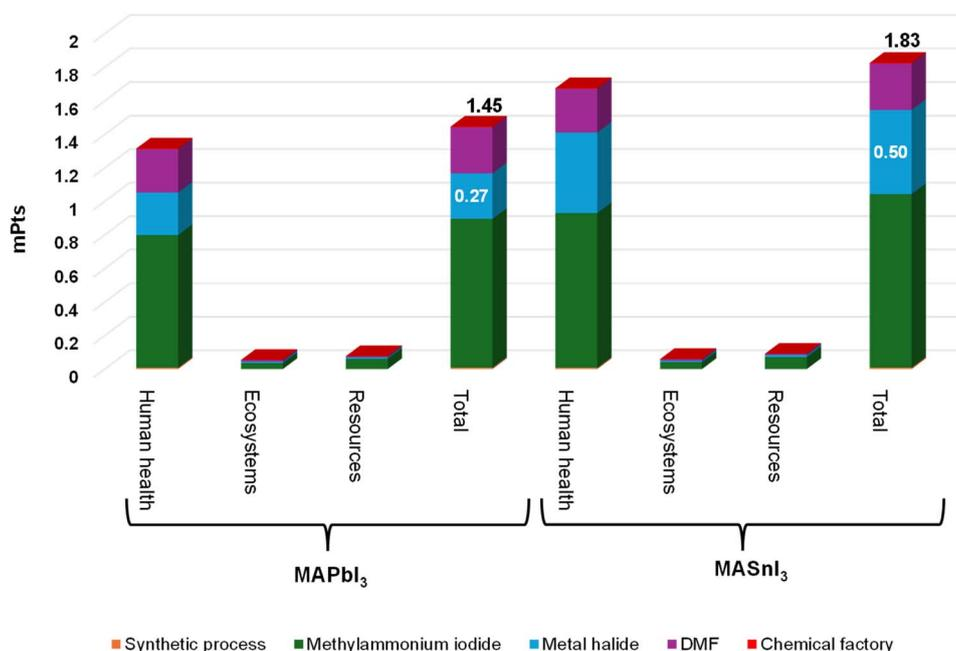
Fig. 4 Endpoint single score (mPts) characterization for the synthesis of 1 g of MAPbI<sub>3</sub> and MASnI<sub>3</sub> (40 wt% in DMF). Focus of the component contribution into the three damage areas.
