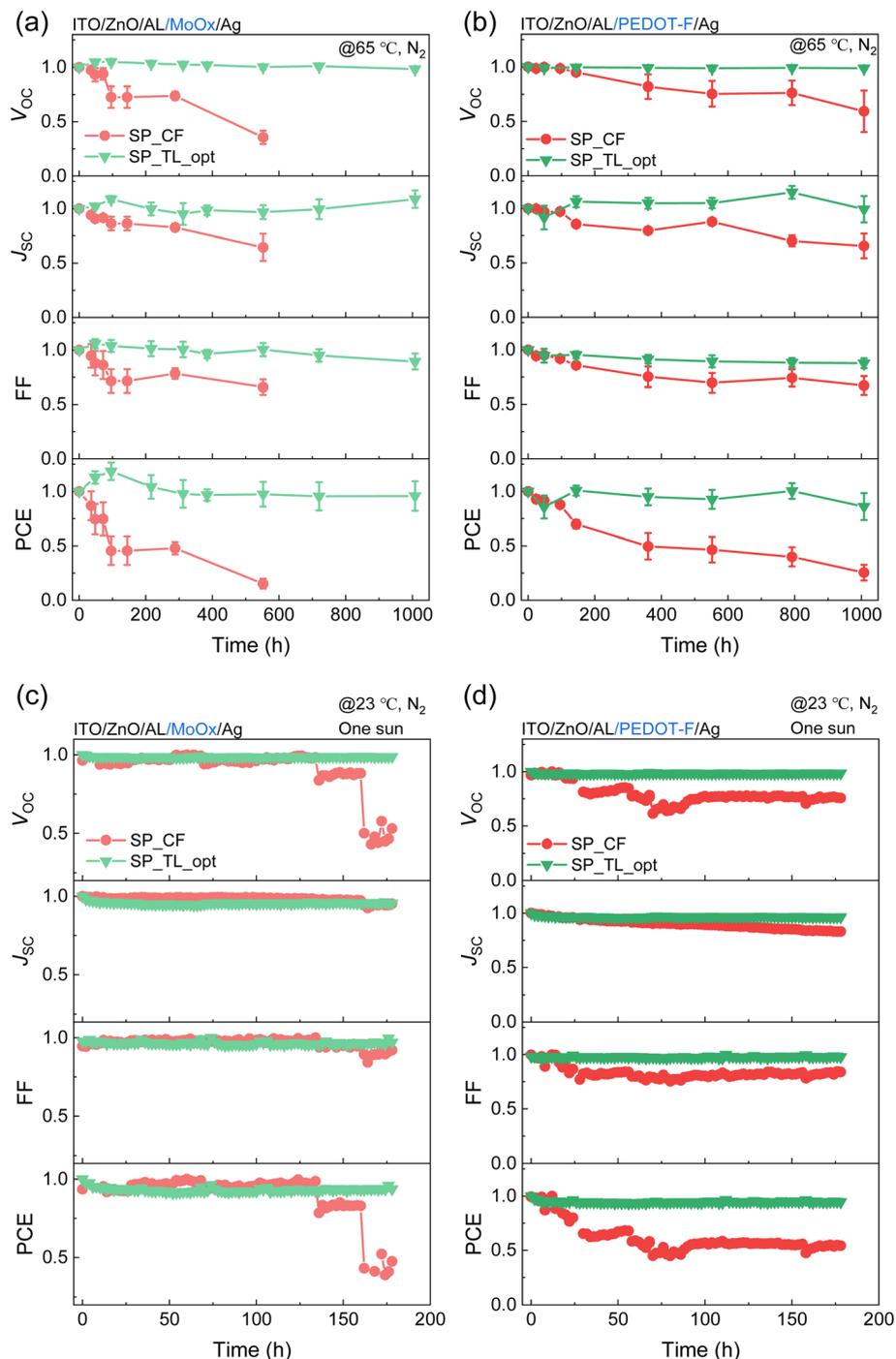
Fig. 4 The thermal and photostability of SP\_CF and SP\_TL\_opt devices fabricated with two different device architectures: ITO/ZnO/active layer/MoO<sub>x</sub>/Ag and ITO/ZnO/active layer/PEDOT-F/Ag. (a and b) Thermal stability was evaluated under continuous thermal aging at 65 °C under a dry nitrogen atmosphere without encapsulation. (c and d) Photostability was assessed under continuous one-sun illumination at 23 °C under a dry nitrogen atmosphere without encapsulation.
