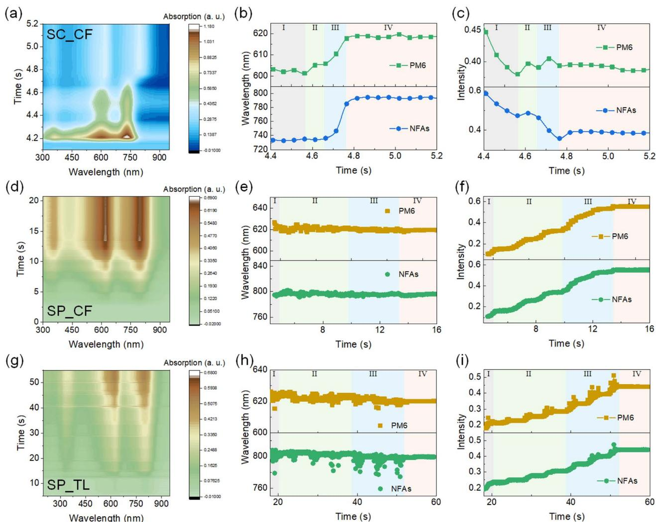
Fig. 2 (a–c) *In situ* UV-vis 2D mapping of the film formation kinetics for SC\_CF, SP\_CF and SP\_TL, respectively. (d–f) Primary peak positions and (g–i) the corresponding normalized peak intensities of SC\_CF, SP\_CF and SP\_TL during the *in situ* experiment.
