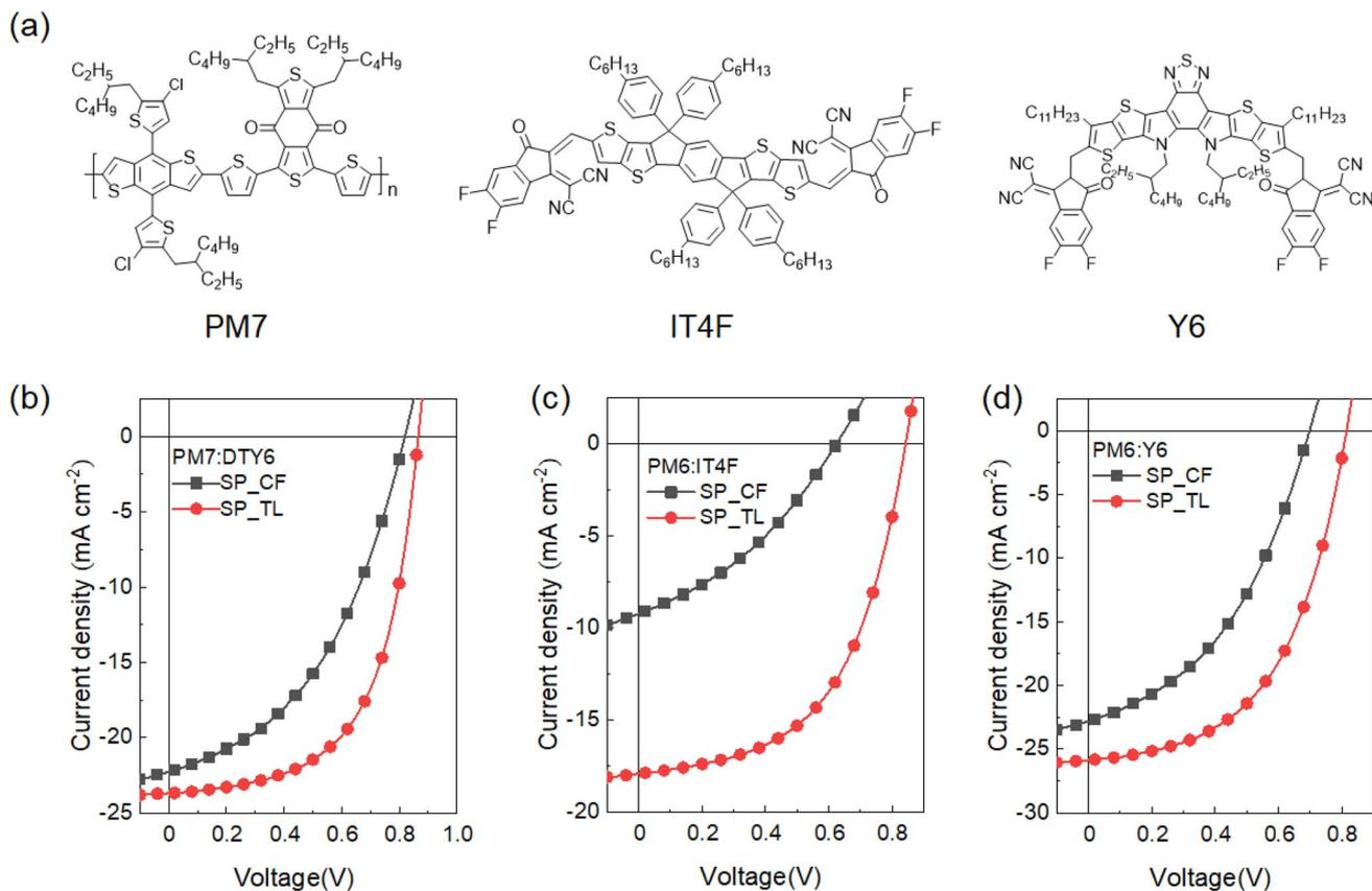
Fig. 5 (a) Chemical structures of PM7, IT4F and Y6 employed in this study. (b–d)  $J$ – $V$  characteristics for the OSCs with spray coating with PM7 : DTY6, PM6 : IT4F and PM6 : Y6 with CF and TL solvent.
