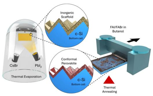
Fig. 1 Schematic illustrating the hybrid evaporation/blade-coating route for scalable perovskite film manufacturing on textured silicon solar cells. The blade-coating step is carried out in the glovebox and the thermal annealing step is carried out after that in air.
