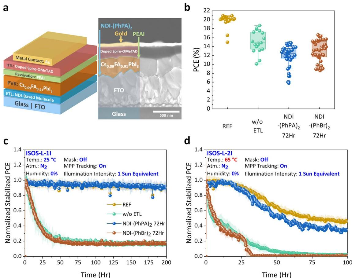
Fig. 4 Photovoltaic performance of NDI-based ETLs in PSCs. (a) Schematic and cross-sectional SEM image of the n-i-p PSC device configuration and (b) PCE from reverse  $J-V$  scans. Long-term stability of PSCs under constant simulated AM 1.5G illumination and MPPT in continuous N<sub>2</sub> flow at (c) 25 °C and (d) 65 °C. "REF" refers to PSCs with c-TiO<sub>2</sub> + mp-TiO<sub>2</sub> as the control ETL, while "w/o ETL" represents devices without an ETL.
