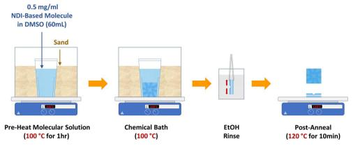
Fig. 2 CBD process of NDI-based ETLs. Schematic representation of the CBD process of NDI-based thin films
