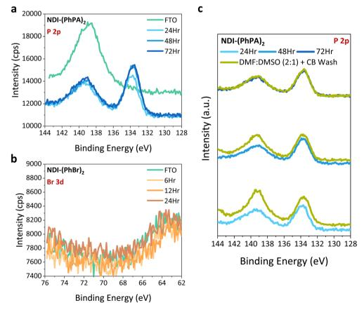
Fig. 3 XPS analysis of NDI-based ETLs on FTO. XPS spectra of (a) P 2p for NDI-(PhPA)<sub>2</sub> and (b) Br 3d for NDI-(PhBr)<sub>2</sub>, deposited on FTO substrates under varying chemical bath durations. (c) XPS spectra of P 2p for NDI-(PhPA)<sub>2</sub> on FTO substrate, before and after washing with DMF: DMSO (2: 1) and CB solvents, simulating the perovskite spin-coating conditions to assess molecular retention.
