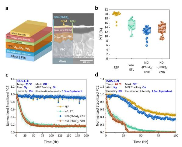
Fig. 4 Photovoltaic performance of NDI-based ETLs in PSCs. (a) Schematic and cross-sectional SEM image of the n-i-p PSC device configuration and (b) PCE from reverse J-V scans. Long-term stability of PSCs under constant simulated AM 1.5G illumination and MPPT in continuous  $N_2$  flow at (c) 25 °C and (d) 65 °C. "REF" refers to PSCs with  $c-TiO_2 + mp-TiO_2$  as the control ETL, while "w/o ETL" represents devices without an ETL.
