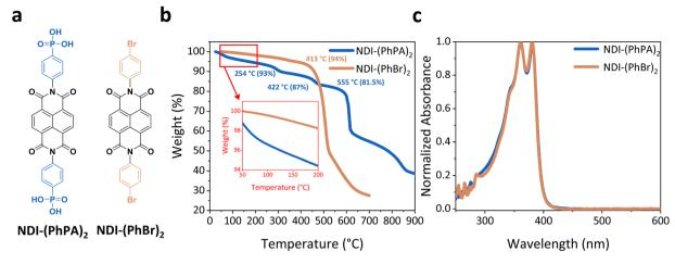
Fig. 1 Molecular structure, thermal stability, and optical property of NDI-based ETLs. (a) Molecular structure, (b) thermogram, and (c) normalized solution UV-vis absorption spectra of NDI-(PhPA)2 and NDI-(PhBr)2 molecules.
