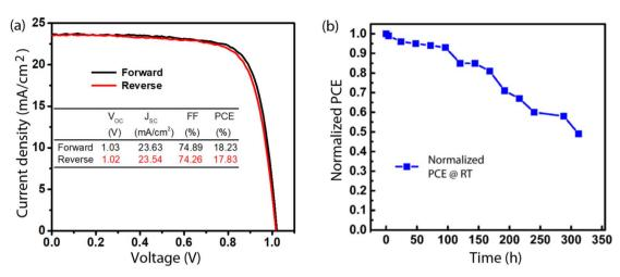
Fig. 6 Photovoltaic performance of the champion perovskite solar cells. (a) Current density vs. voltage (J-V) curve. (b) Efficiency evolution of the unencapsulated device (a) exposed in ambient air with a relative humidity (RH) of  $\sim$ 60  $\pm$ 8%.
