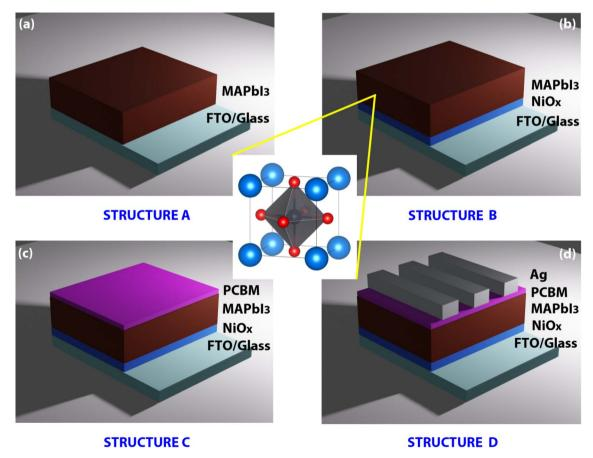
Fig. 1 Schematics of four different device structures for investigating the humid-air stress effect on the stability of perovskite solar cells: (a) structure A: FTO/MAPbl<sub>3</sub>, (b) structure B: FTO/NiO<sub>x</sub>/MAPbl<sub>3</sub>, (c) structure C: FTO/NiO<sub>x</sub>/MAPbl<sub>3</sub>/PCBM and (d) structure D: FTO/NiO<sub>x</sub>/MAPbl<sub>3</sub>/ PCBM/Ag. (Inset) The unit cell of MAPbI<sub>3</sub> perovskite.
