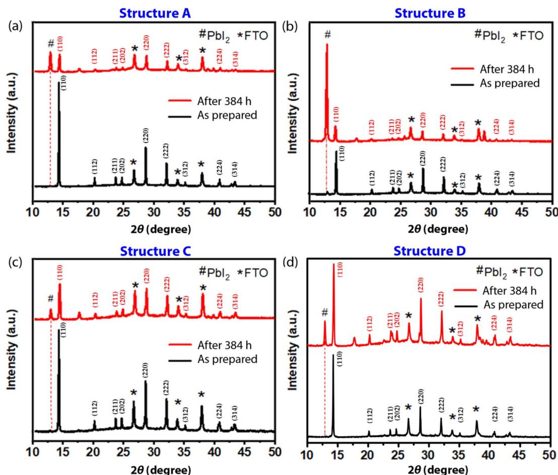
Fig. 5 XRD patterns of unencapsulated fresh samples and those after 16 days in open air (with a relative humidity of  $\sim 60 \pm 8\%$ ): (a) structure A: FTO/MAPbI<sub>3</sub>, (b) structure B: FTO/NiO<sub>x</sub>/MAPbI<sub>3</sub>, (c) structure C: FTO/NiO<sub>x</sub>/MAPbI<sub>3</sub>/PCBM, and (d) structure D: FTO/NiO<sub>x</sub>/MAPbI<sub>3</sub>/PCBM/Ag.
