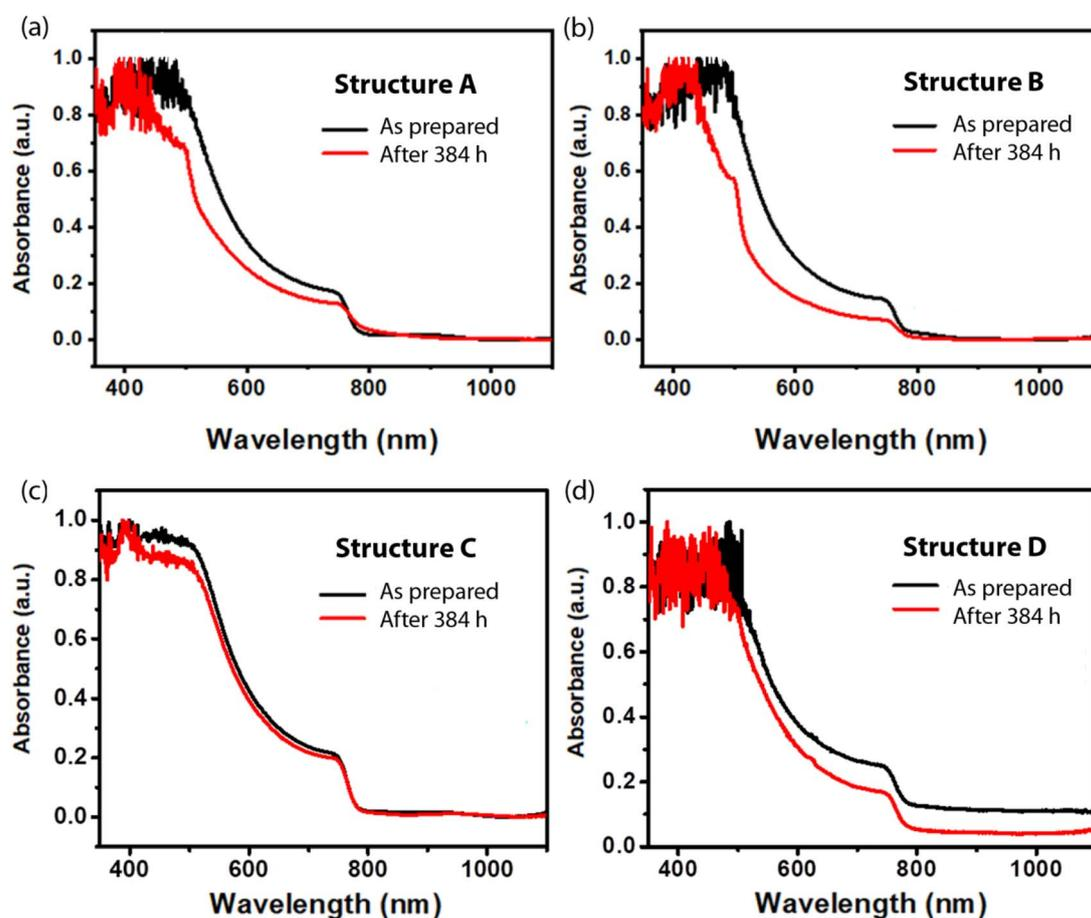
Fig. 4 UV-vis absorption of fresh samples and those after 16 days (=384 h): (a) structure A: FTO/MAPbI<sub>3</sub>, (b) structure B: FTO/NiO<sub>x</sub>/MAPbI<sub>3</sub>, (c) structure C: FTO/NiO<sub>x</sub>/MAPbI<sub>3</sub>/PCBM, and (d) structure D: FTO/NiO<sub>x</sub>/MAPbI<sub>3</sub>/PCBM/Ag. The samples were exposed to oxygen and moisture with a relative humidity of  $\sim 60 \pm 8\%$ .
