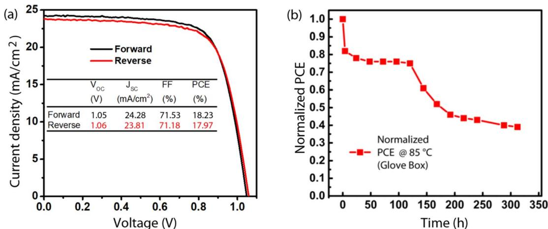
Fig. 10 Photovoltaic performance of perovskite solar cells. (a) Current density vs. voltage ( $J$ - $V$ ) curve of a fresh device. (b) Normalized power conversion efficiency vs. aging time. Here, the unencapsulated devices were exposed to 85 °C in a N<sub>2</sub>-filled glove box.
