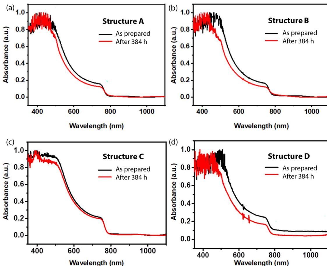
Fig. 8 UV-vis absorption spectra of (a) structure A: FTO/ $MAPbI_3$ , (b) structure B: FTO/ $NiO_x$ /MAPbI<sub>3</sub>, (c) structure C: FTO/ $NiO_x$ /MAPbI<sub>3</sub>/PCBM, and (d) structure D: FTO/ $NiO_x$ /MAPbI<sub>3</sub>/PCBM/Ag. Samples were kept unencapsulated for 12 days at  $85^\circ C$  in a  $N_2$ -filled glove box.
