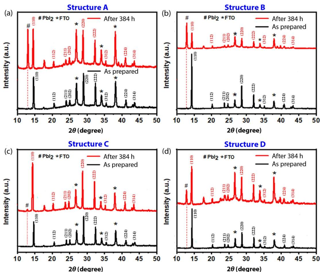
Fig. 9 XRD patterns of (a) structure A: FTO/MAPbI<sub>3</sub>, (b) structure B: FTO/NiO<sub>x</sub>/MAPbI<sub>3</sub>, (c) structure C: FTO/NiO<sub>x</sub>/MAPbI<sub>3</sub>/PCBM, and (d) structure D: FTO/NiO<sub>x</sub>/MAPbI<sub>3</sub>/PCBM/Ag. The samples were kept unencapsulated for 12 days at 85 °C in a glove box.
