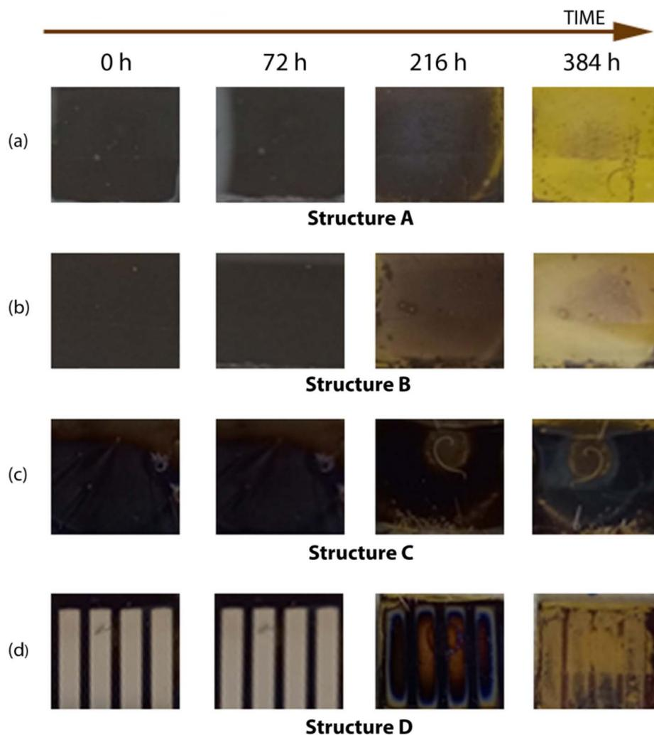
Fig. 2 Photographs showing the stability of (a) structure A: FTO/MAPbI<sub>3</sub>, (b) structure B: FTO/NiO<sub>x</sub>/MAPbI<sub>3</sub>, (c) structure C: FTO/NiO<sub>x</sub>/MAPbI<sub>3</sub>/PCBM, and (d) structure D: FTO/NiO<sub>x</sub>/MAPbI<sub>3</sub>/PCBM/Ag as a function of storage time in air with a relative humidity of  $\sim 60 \pm 8\%$ . The FTO substrate size was  $1.8 \times 1.5$  cm<sup>2</sup>.
