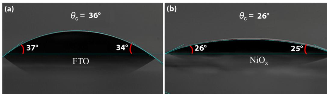
Fig. 3 Water contact angle on (a) FTO and (b) NiO<sub>x</sub> layers, respectively.
