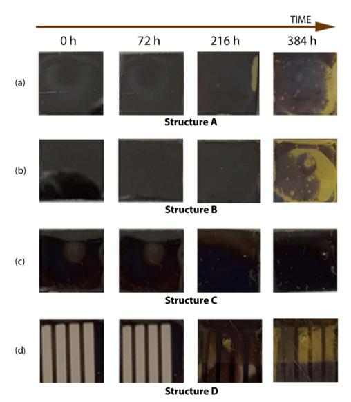
Fig. 7 Photographs of (a) structure A: FTO/MAPbl<sub>3</sub>, (b) structure B: FTO/NiO<sub>x</sub>/MAPbl<sub>3</sub>, (c) structure C: FTO/NiO<sub>x</sub>/MAPbl<sub>3</sub>/PCBM, and (d) structure D: FTO/NiO<sub>x</sub>/MAPbl<sub>3</sub>/PCBM/Ag. Samples were kept unencapsulated for 16 days at 85 °C inside a nitrogen-filled glove box. The FTO substrate size is  $1.8 \times 1.5 \text{ cm}^2$ .
