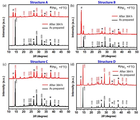
Fig. 5 XRD patterns of unencapsulated fresh samples and those after 16 days in open air (with a relative humidity of  $\sim$ 60  $\pm$  8%): (a) structure A: FTO/MAPbl<sub>3</sub>, (b) structure B: FTO/NiO<sub>4</sub>/MAPbl<sub>3</sub>, (c) structure C: FTO/NiO<sub>4</sub>/MAPbl<sub>3</sub>/PCBM, and (d) structure D: FTO/NiO<sub>4</sub>/MAPbl<sub>3</sub>/PCBM/Ag.
