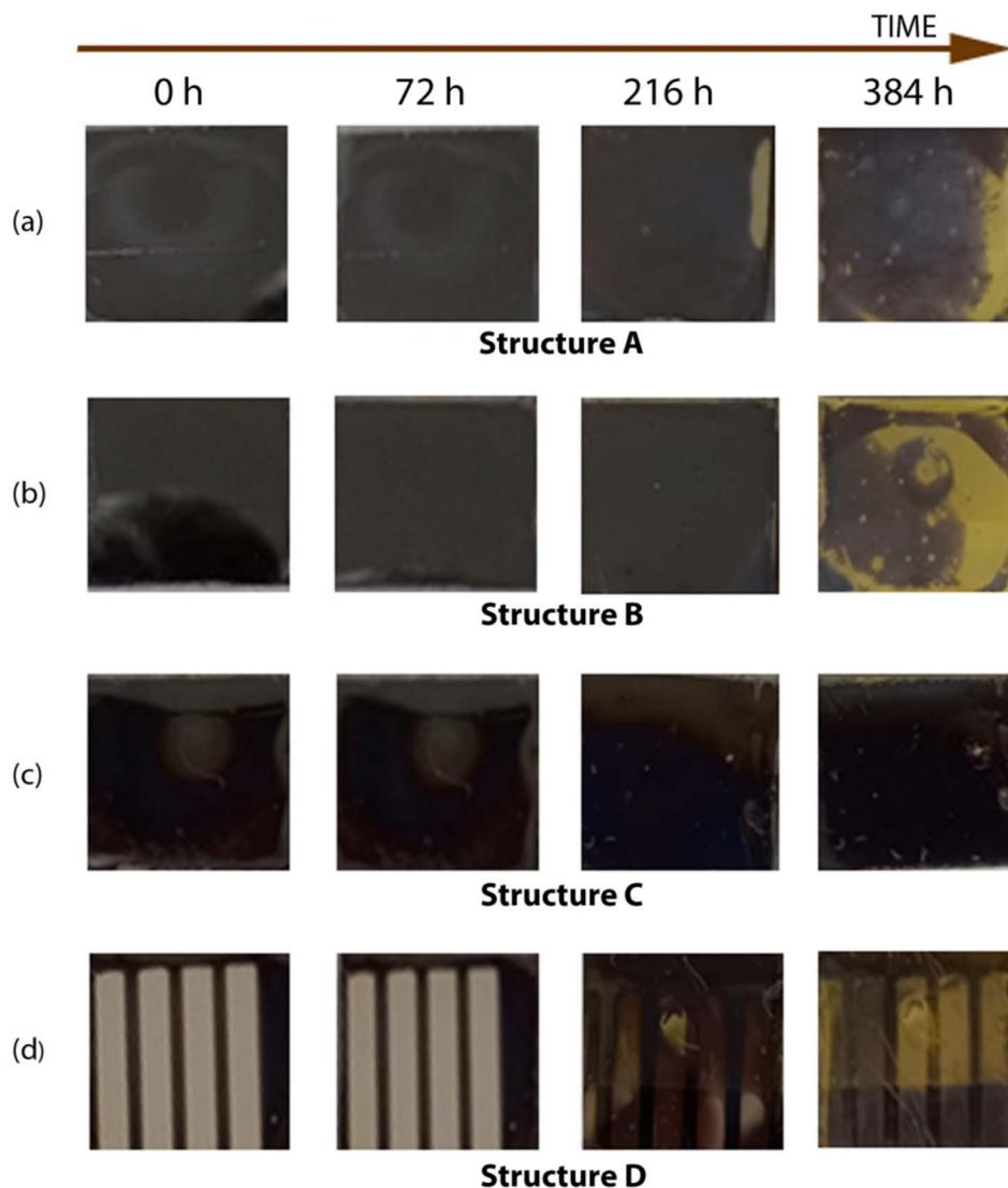
Fig. 7 Photographs of (a) structure A: FTO/MAPbI<sub>3</sub>, (b) structure B: FTO/NiO<sub>x</sub>/MAPbI<sub>3</sub>, (c) structure C: FTO/NiO<sub>x</sub>/MAPbI<sub>3</sub>/PCBM, and (d) structure D: FTO/NiO<sub>x</sub>/MAPbI<sub>3</sub>/PCBM/Ag. Samples were kept unencapsulated for 16 days at 85 °C inside a nitrogen-filled glove box. The FTO substrate size is  $1.8 \times 1.5 \text{ cm}^2$ .
