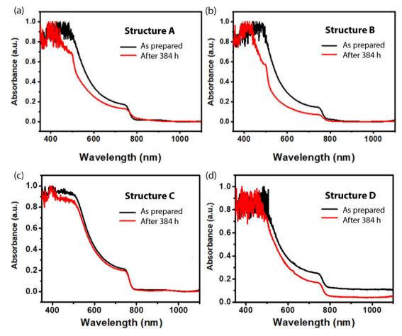
Fig. 4 UV-vis absorption of fresh samples and those after 16 days (=384 h): (a) structure A: FTO/MAPbl<sub>3</sub>, (b) structure B: FTO/NiO<sub>x</sub>/MAPbl<sub>3</sub>, (c) structure C: FTO/NiO<sub>x</sub>/MAPbI<sub>3</sub>/PCBM, and (d) structure D: FTO/NiO<sub>x</sub>/MAPbI<sub>3</sub>/PCBM/Ag. The samples were exposed to oxygen and moisture with a relative humidity of  $\sim$ 60  $\pm$  8%.
