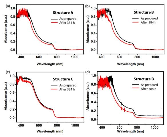
Fig. 8 UV-vis absorption spectra of (a) structure A: FTO/MAPbl<sub>3</sub>, (b) structure B: FTO/NiO<sub>x</sub>/MAPbl<sub>3</sub>, (c) structure C: FTO/NiO<sub>x</sub>/MAPbl<sub>3</sub>/PCBM, and (d) structure D: FTO/NiO<sub>x</sub>/MAPbI<sub>x</sub>/PCBM/Aq. Samples were kept unencapsulated for 12 days at 85 °C in a N<sub>2</sub>-filled glove box.
