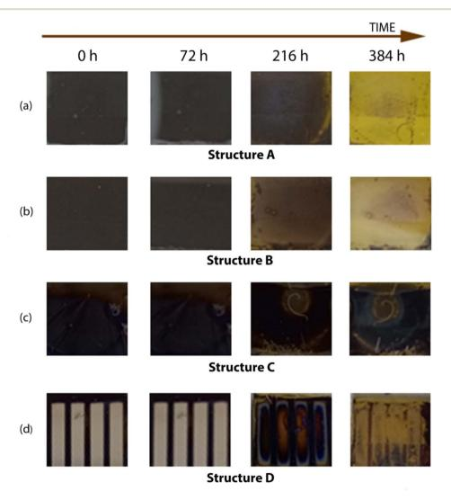
Fig. 2 Photographs showing the stability of (a) structure A: FTO/MAPbI<sub>3</sub>, (b) structure B: FTO/NiO<sub>x</sub>/MAPbI<sub>3</sub>, (c) structure C: FTO/NiO<sub>x</sub>/MAPbI<sub>3</sub>, PCBM, and (d) structure D: FTO/NiO<sub>x</sub>/MAPbl<sub>3</sub>/PCBM/Aq as a function of storage time in air with a relative humidity of  $\sim$ 60  $\pm$  8%. The FTO substrate size was  $1.8 \times 1.5$  cm<sup>2</sup>.
