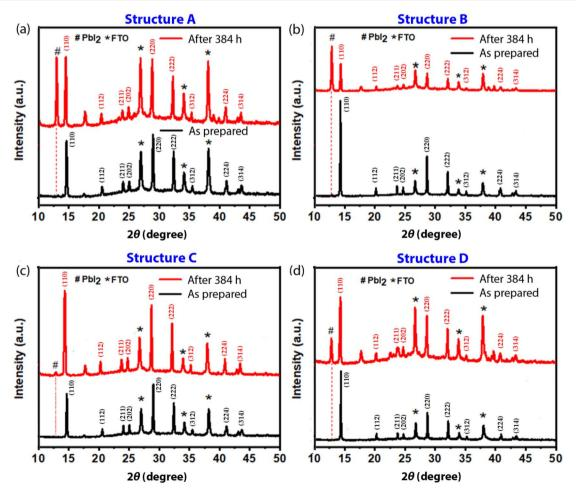
Fig. 9 XRD patterns of (a) structure A: FTO/MAPbl<sub>3</sub>, (b) structure B: FTO/NiO<sub>x</sub>/MAPbl<sub>3</sub>, (c) structure C: FTO/NiO<sub>x</sub>/MAPbl<sub>3</sub>/PCBM, and (d) structure D: FTO/NiO<sub>x</sub>/MAPbl<sub>3</sub>/PCBM/Ag. The samples were kept unencapsulated for 12 days at 85 °C in a glove box.
