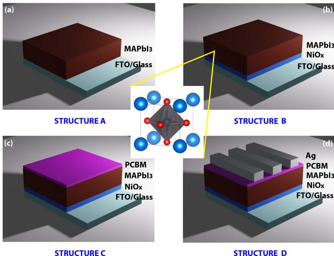
Fig. 1 Schematics of four different device structures for investigating the humid-air stress effect on the stability of perovskite solar cells: (a) structure A: FTO/MAPbI<sub>3</sub>, (b) structure B: FTO/NiO<sub>x</sub>/MAPbI<sub>3</sub>, (c) structure C: FTO/NiO<sub>x</sub>/MAPbI<sub>3</sub>/PCBM and (d) structure D: FTO/NiO<sub>x</sub>/MAPbI<sub>3</sub>/PCBM/Ag. (Inset) The unit cell of MAPbI<sub>3</sub> perovskite.
