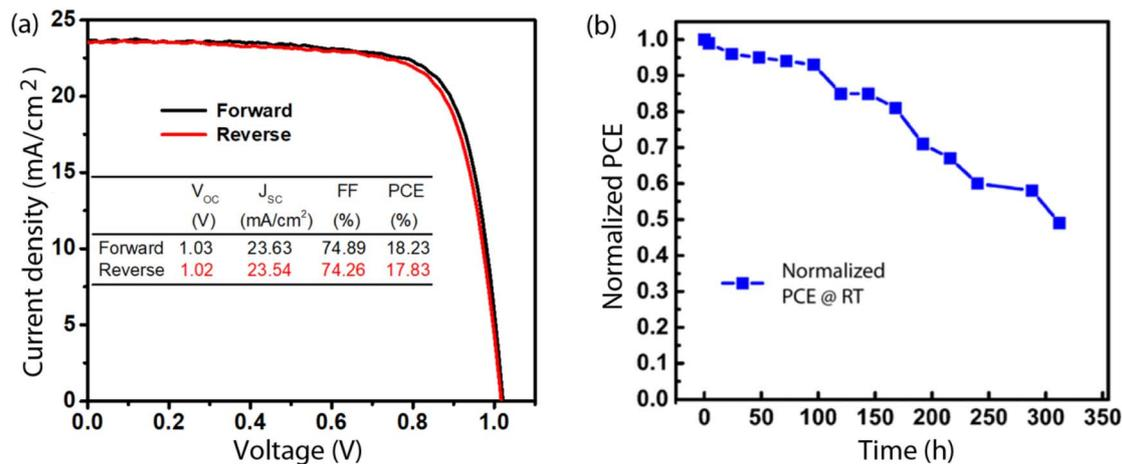
Fig. 6 Photovoltaic performance of the champion perovskite solar cells. (a) Current density vs. voltage ( $J$ - $V$ ) curve. (b) Efficiency evolution of the unencapsulated device (a) exposed in ambient air with a relative humidity (RH) of  $\sim 60 \pm 8\%$ .
