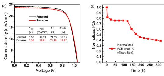
Fig. 10 Photovoltaic performance of perovskite solar cells. (a) Current density vs. voltage (J-V) curve of a fresh device. (b) Normalized power conversion efficiency vs. aging time. Here, the unencapsulated devices were exposed to 85 °C in a  $N_2$ -filled glove box.
