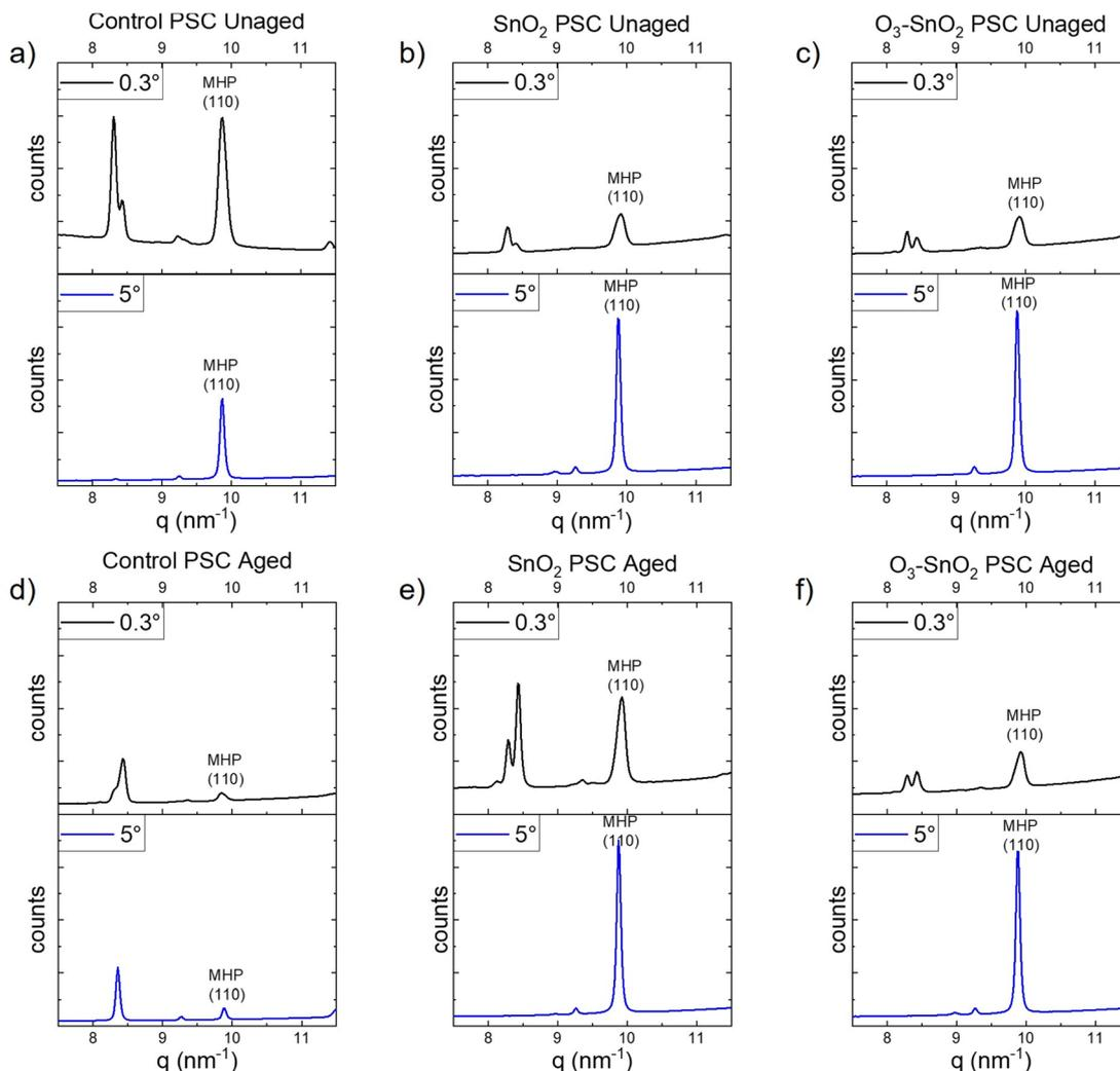
Fig. 4 Improved bulk MHP stability of PSCs with barrier layer X-ray diffraction plots in  $q$ -space at incidence angles  $0.3^\circ$  (representing the top surface) and  $5^\circ$  (representing the bulk) (a–c) unaged PSCs, and (d–f) PSCs subjected to  $50^\circ\text{C}$  for 120 h. (a and d) Control PSC, (b and e)  $\text{SnO}_2$  PSC, and (c and f)  $\text{O}_3\text{-SnO}_2$  PSC.
