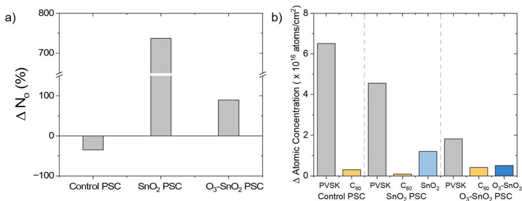
Fig. 2 Effectiveness of SnO<sub>2</sub> barrier layer in the prevention of Ag ion diffusion (a) percentage change in  $N_0$  for control PSC, SnO<sub>2</sub> PSC, and O<sub>3</sub>-SnO<sub>2</sub> PSC with Ag top electrodes after exposure of the PSCs to 50 °C for 120 h. (b) Change in RBS atomic concentration of Ag after aging in the MHP layer and ETL for control PSC, along with barrier layer for SnO<sub>2</sub> PSC, and O<sub>3</sub>-SnO<sub>2</sub> PSC.
