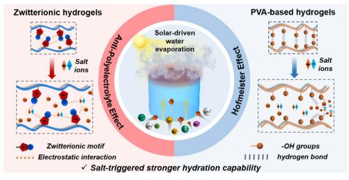
Fig. 1 Schematic illustration of the salt ion triggered hydration chemistry for salt-rejecting solar-driven water evaporation.
