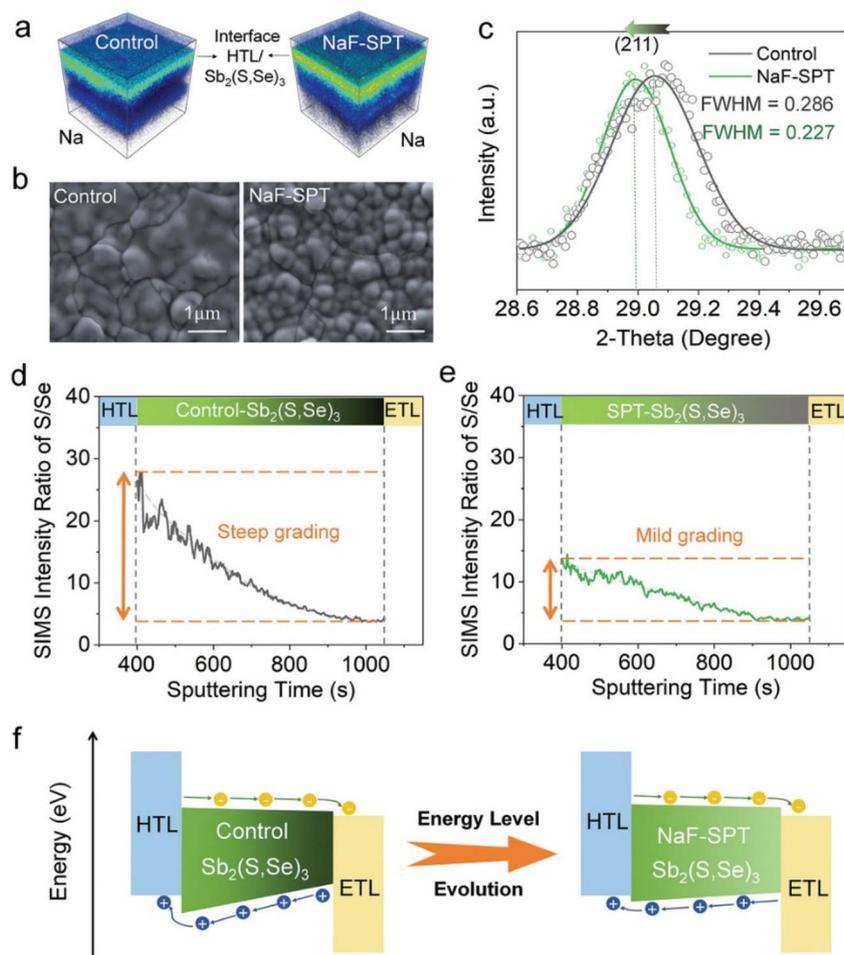
Fig. 3 (a) 3D-SIMS images of Na. (b) Surface SEM images. (c) Enlarged XRD spectra of 2-theta from 28.6° to 29.8°. (d and e) SIMS intensity ratios of S/Se in  $\text{Sb}_2(\text{S,Se})_3$  films. (f) Schematic diagram of energy levels of  $\text{Sb}_2(\text{S,Se})_3$  devices with or without NaF-SPT. Reproduced with permission from ref. 27 with permission from Wiley, copyright 2022.
