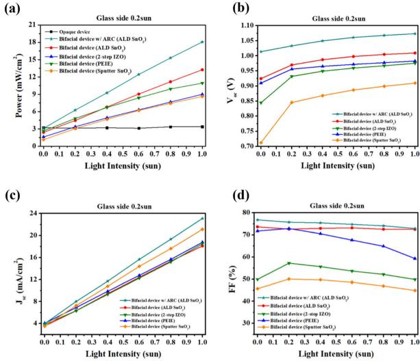
Fig. 14 (a) Power output density, (b)  $V_{oc}$ , (c)  $J_{sc}$ , and (d) FF of different bifacial devices under fixed 0.2 sun illumination on the glass side (approaching rainy day intensity) with varying light intensities from the IZO side.
