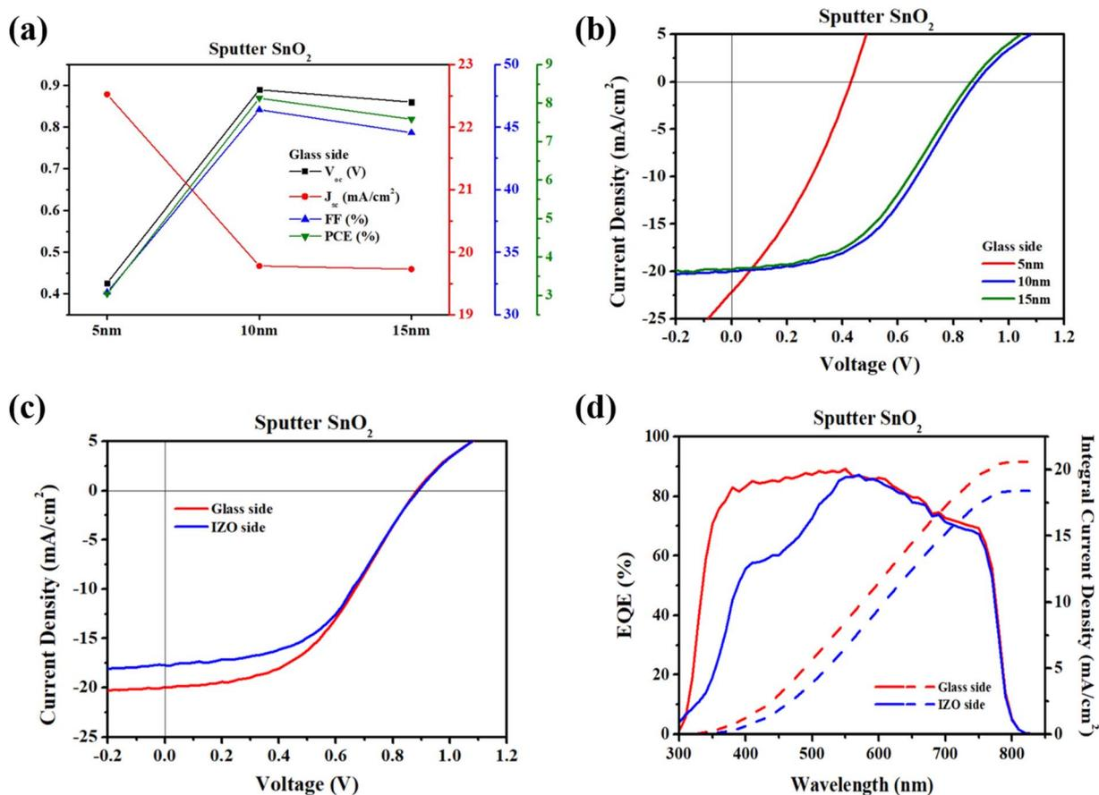
Fig. 4 (a) PV parameters and (b)  $J$ - $V$  curves of the bifacial devices with different sputtered-buffer  $\text{SnO}_2$  thicknesses under AM 1.5 G illumination through the FTO substrate. (c)  $J$ - $V$  curves and (d) EQE spectra for 10 nm  $\text{SnO}_2$  devices under front and rear illumination.
