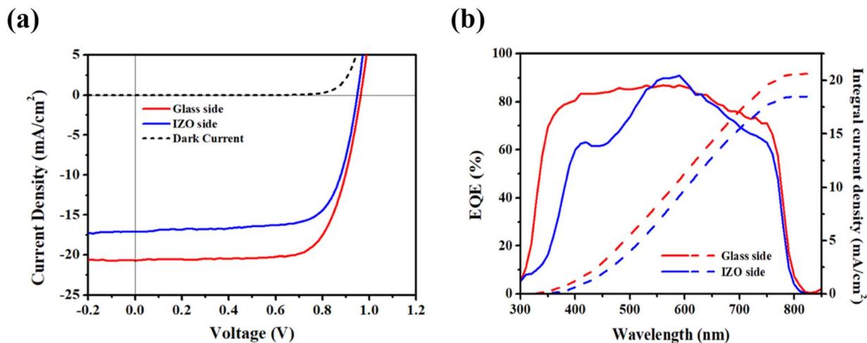
Fig. 8 (a)  $J$ - $V$  curve and (b) EQE spectra of the ALD  $\text{SnO}_2$  10 nm bifacial device under 1 sun illumination from glass and IZO sides.
