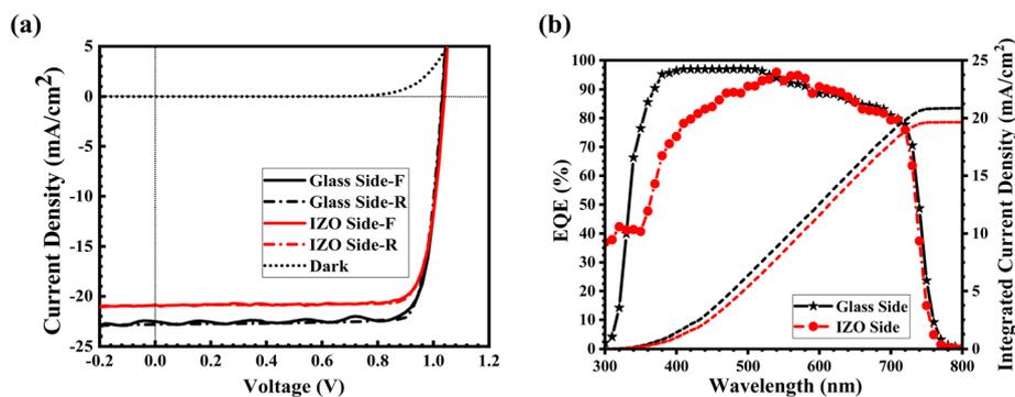
Fig. 15 (a)  $J$ - $V$  curve and (b) EQE spectra of the MA free perovskite (FA<sub>0.78</sub>CS<sub>0.22</sub>Pb(I<sub>0.85</sub>Br<sub>0.15</sub>)<sub>3</sub>) bifacial device under 1 sun illumination from glass and IZO sides.
