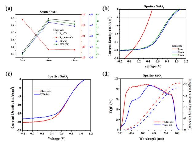
Fig. 4 (a) PV parameters and (b) J-V curves of the bifacial devices with different sputtered-buffer SnO<sub>2</sub> thicknesses under AM 1.5 G illumination through the FTO substrate. (c) J-V curves and (d) EQE spectra for 10 nm  $SnO_2$  devices under front and rear illumination
