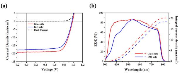
(a) J-V curve and (b) EQE spectra of the bifacial device with 0.4 wt% PEIE under 1 sun illumination from glass and IZO sides.
