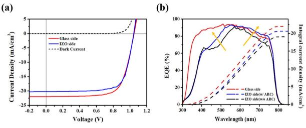
Fig. 9 (a) J-V curves and (b) EQE spectra of ALD SnO<sub>2</sub> bifacial device with an ARC illuminated with 1 sun from glass and IZO sides.
