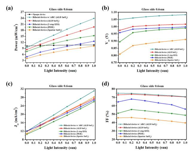
Fig. 13 (a) Power output density, (b)  $V_{\text{OC}}$ , (c)  $J_{\text{SC}}$ , and (d) FF of different bifacial devices under fixed 0.6 sun illumination on the glass side (approaching cloudy day intensity) with varying light intensities from the IZO side.
