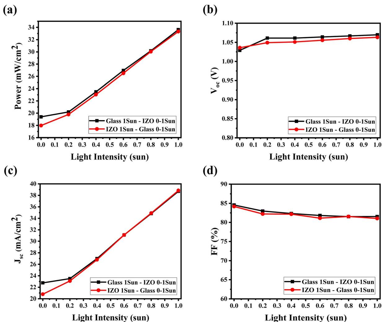
Fig. 16 (a) Power output and (b)  $V_{oc}$  (c) photocurrent and (d) FF of the MA free perovskite ( $\text{FA}_{0.78}\text{Cs}_{0.22}\text{Pb}(\text{I}_{0.85}\text{Br}_{0.15})_3$ ) bifacial illuminated device as a function of backside illumination intensities with fixed 1 sun intensity from glass (blackline) and IZO (red line) sides.
