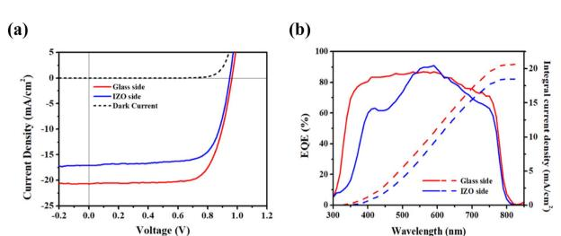
Fig. 8 (a) J-V curve and (b) EQE spectra of the ALD SnO<sub>2</sub> 10 nm bifacial device under 1 sun illumination from glass and IZO sides.
