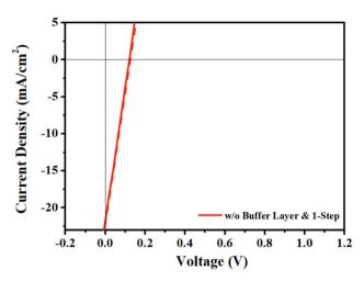
Fig. 2 The  $J\!-\!V$  curves of the bifacial device where the IZO film is directly deposited on the  $C_{60}$  layer without any buffer layer.
