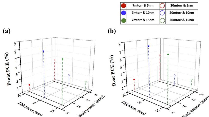
Fig. 5 For bifacial devices with sputtered buffer layers, measured under AM 1.5 G 1 sun illumination, the performance with different SnO<sub>2</sub> thicknesses and working pressures: (a) front-side efficiency and (b) rear-side efficiency.
