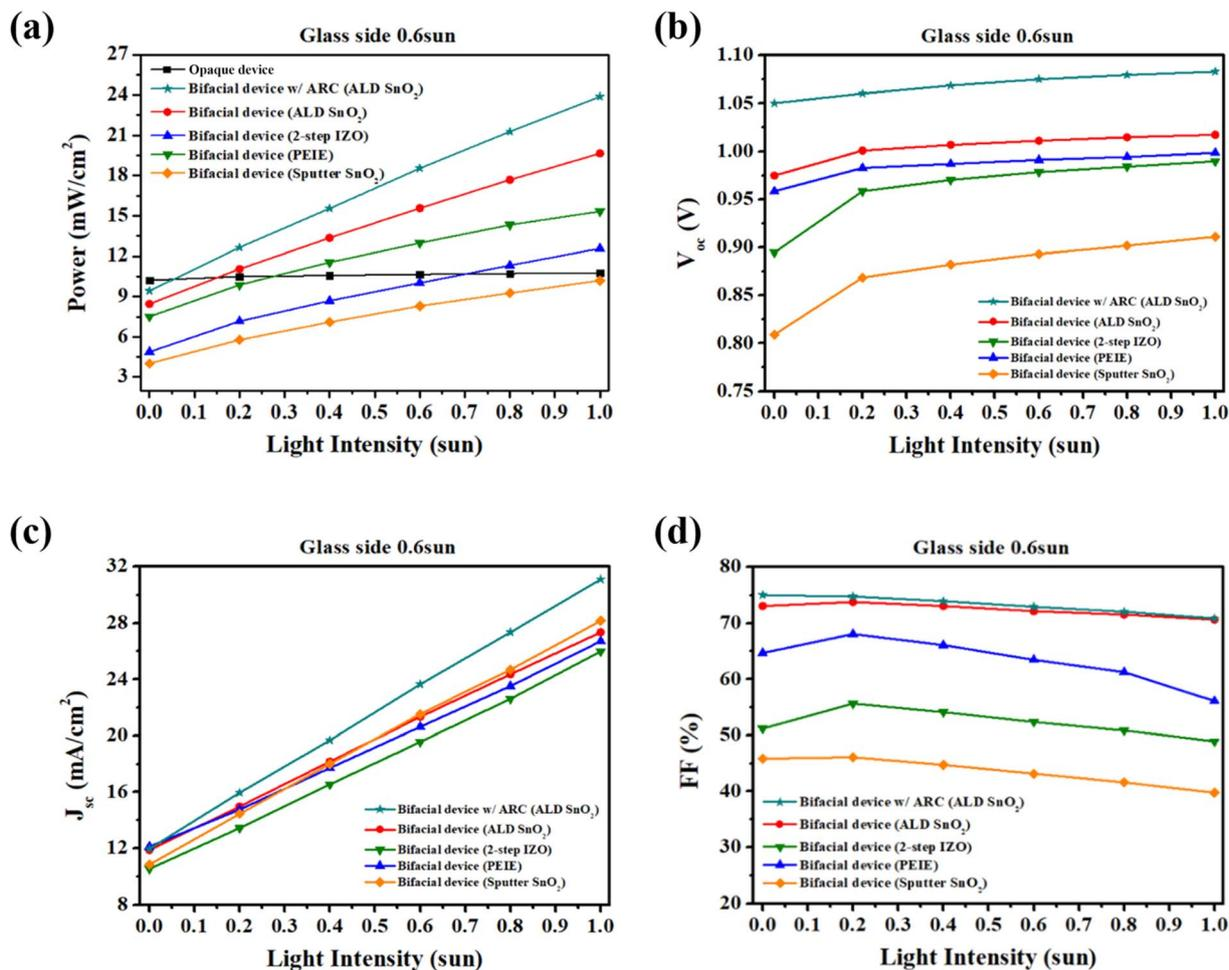
Fig. 13 (a) Power output density, (b)  $V_{oc}$ , (c)  $J_{sc}$ , and (d) FF of different bifacial devices under fixed 0.6 sun illumination on the glass side (approaching cloudy day intensity) with varying light intensities from the IZO side.
