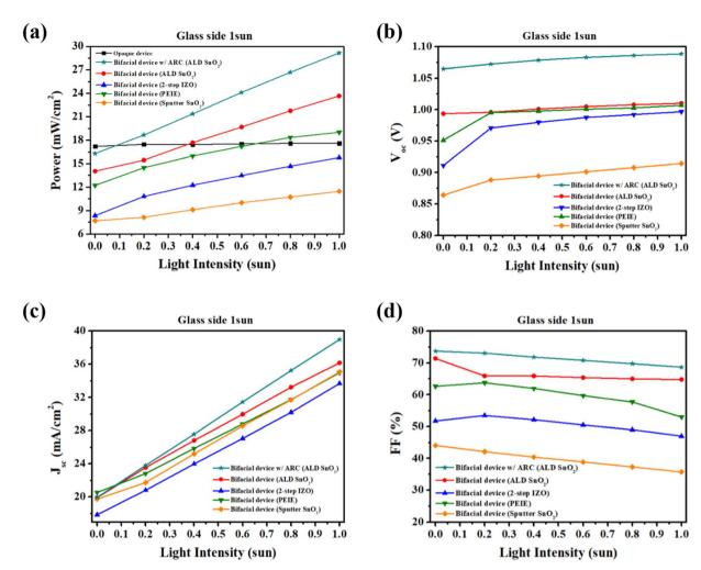
Fig. 12 (a) Power output density, (b)  $V_{oc}$ , (c)  $J_{sc}$ , and (d) FF of different bifacial devices under fixed 1 sun illumination on the glass side (approaching sunny day intensity) with varying light intensities from the IZO side.
