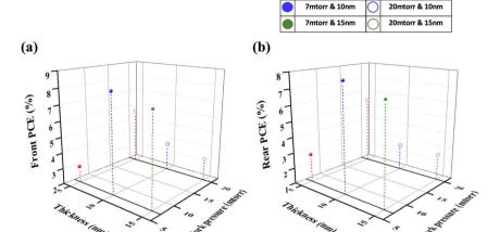
Fig. 5 For bifacial devices with sputtered buffer layers, measured under AM 1.5 G 1 sun illumination, the performance with different SnO<sub>2</sub> thicknesses and working pressures: (a) front-side efficiency and (b) rear-side efficiency.
