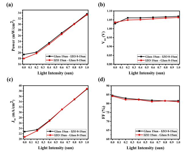
Fig. 16 (a) Power output and (b)  $V_{oc}$  (c) photocurrent and (d) FF of the MA free perovskite (FA<sub>0.78</sub>Cs<sub>0.22</sub>Pb(I<sub>0.85</sub>Br<sub>0.15</sub>)<sub>3</sub>) bifacial illuminated device as a function of backside illumination intensities with fixed 1 sun intensity from glass (blackline) and IZO (red line) sides.
