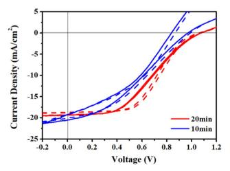
Fig. 3 The J-V curves (solid: forward scan and dashed: reverse scan) for bifacial devices fabricated with different soft deposition times of IZO in the first step of the 2-step IZO process under AM 1.5 G illumination.
