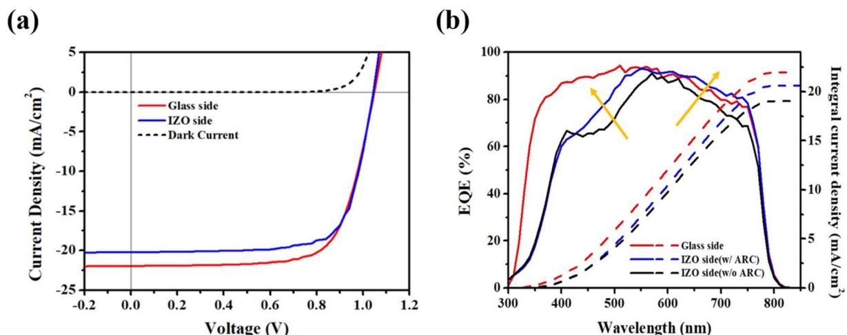
Fig. 9 (a)  $J$ - $V$  curves and (b) EQE spectra of ALD  $\text{SnO}_2$  bifacial device with an ARC illuminated with 1 sun from glass and IZO sides.
