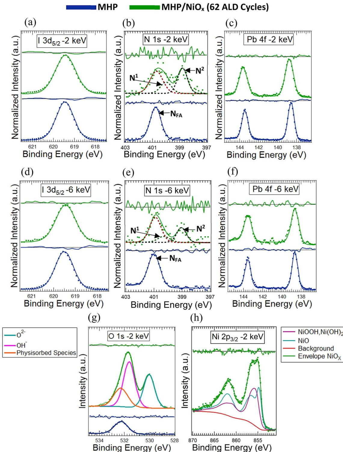
Fig. 2 (a–h) HAXPES detail spectra (including fits and residua) of the (a and d) I 3d<sub>5/2</sub>, (b and e) N 1s, (c and f) Pb 4f, (g) O 1s, and (h) Ni 2p<sub>3/2</sub> core levels of MHP without (blue spectra) and with (green spectra) 62 ALD cycle NiO<sub>x</sub> top layers recorded with (a–c, g and h) 2 keV and (d–f) 6 keV photon energies.
