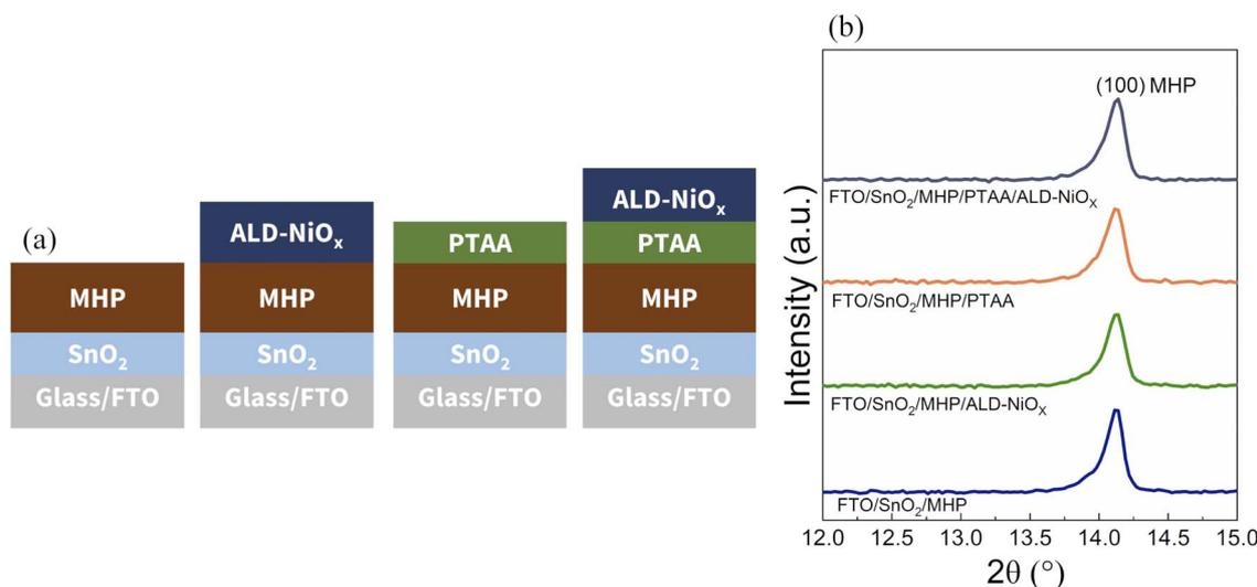
Fig. 1 (a) Schematic of the different device architectures used in this section for interface study, (b) XRD patterns of MHP film with and without ALD- $\text{NiO}_x$ , PTAA, PTAA/ALD- $\text{NiO}_x$  top layers.
