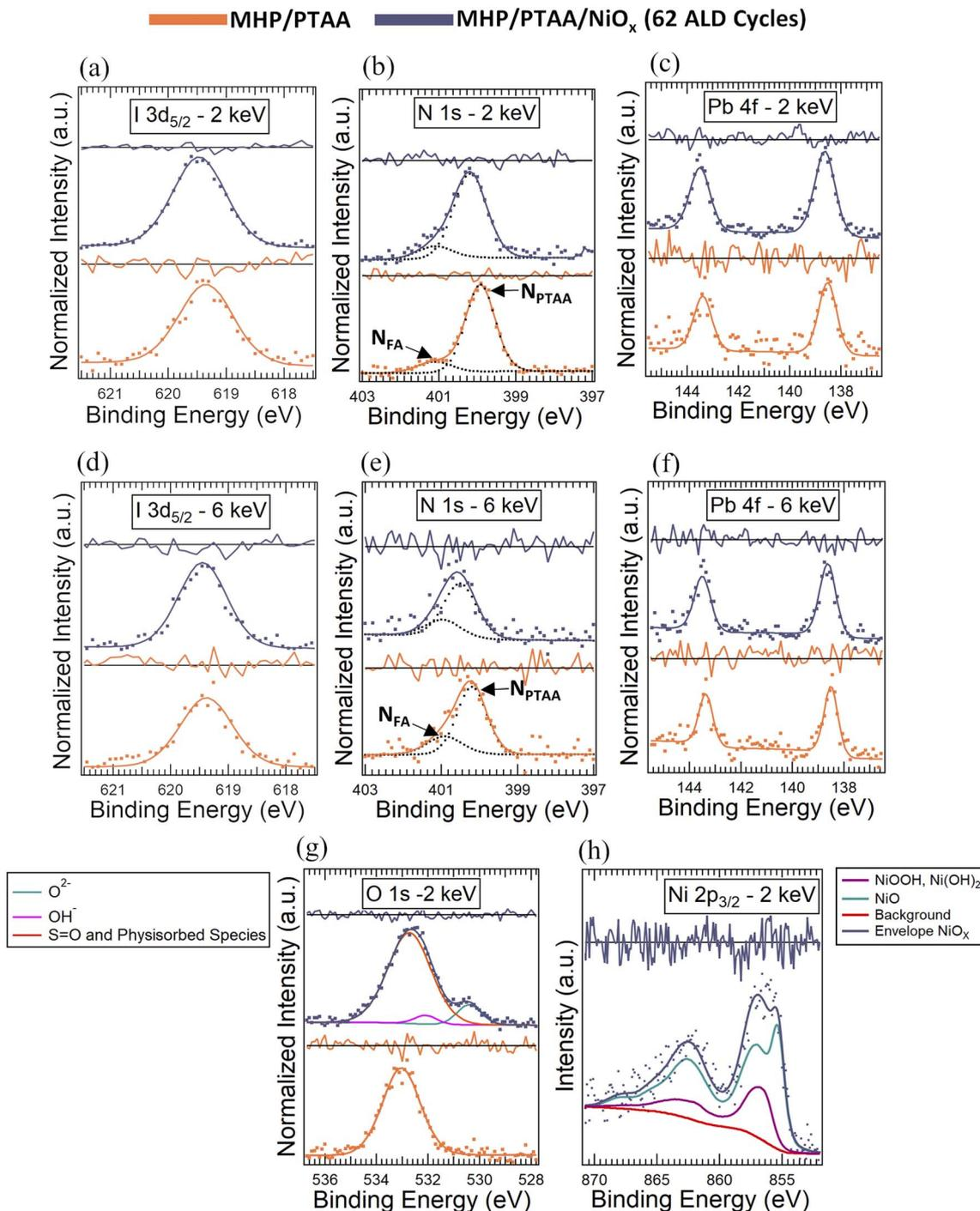
Fig. 4 (a–h) HAXPES detail spectra (including fits and residua) of I  $3d_{5/2}$ , N 1s, Pb 4f, O 1s, Ni  $2p_{3/2}$  of MHP: PTAA without (orange spectra) and with (purple spectra) ALD- $\text{NiO}_x$  top layers recorded with 2 keV and 6 keV excitation energy.
