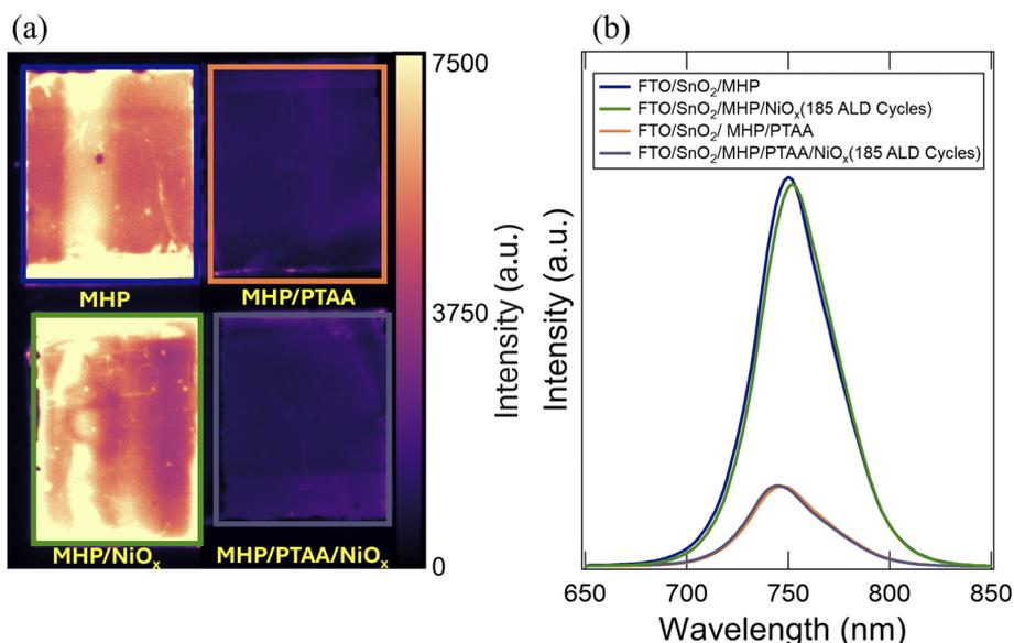
Fig. 6 (a) Hyperspectral photoluminescence (PL) images at 750 nm for FTO/SnO<sub>2</sub>/FA<sub>0.83</sub>CS<sub>0.17</sub>Pb(I<sub>0.83</sub>Br<sub>0.17</sub>)<sub>3</sub> MHP, FTO/SnO<sub>2</sub>/MHP/NiO<sub>x</sub>, FTO/SnO<sub>2</sub>/MHP/PTAA, FTO/SnO<sub>2</sub>/MHP/PTAA/NiO<sub>x</sub>, (b) average PL intensity.
