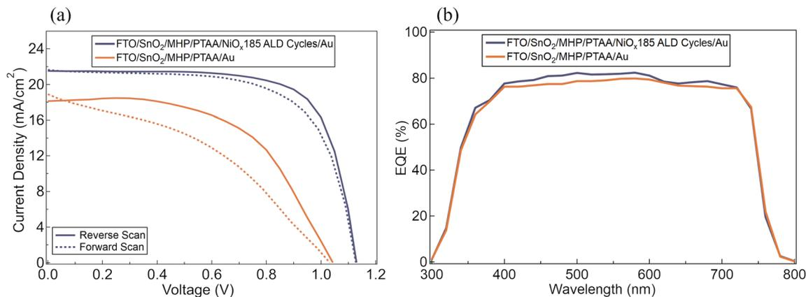
Fig. 5 (a)  $J$ - $V$  characteristics (forward scan shown in solid line and reverse scan shown in dotted line) and (b) external quantum efficiency (EQE) of n-i-p PSCs with and without a 185 ALD cycle NiO<sub>x</sub> overlayer.
