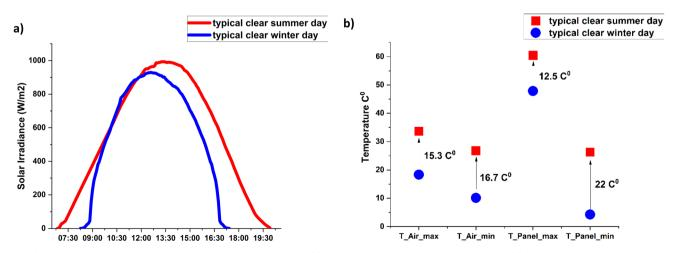
Fig. 5 Comparison between the winter and summer clear days of (a) different irradiation levels and duration. (b) Comparison of maximum air and panel temperature.
