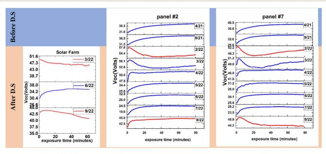
Fig. 6 Light soaking effect behavior change before (4/21 and 8/21) and after the 3-month dark storage (DS) period (2/22) for the solar farm, panel #7, and panel #2, for each month until 9/22. The red color highlights the measurements immediately after the DS periods (2/22 and 9/22)
