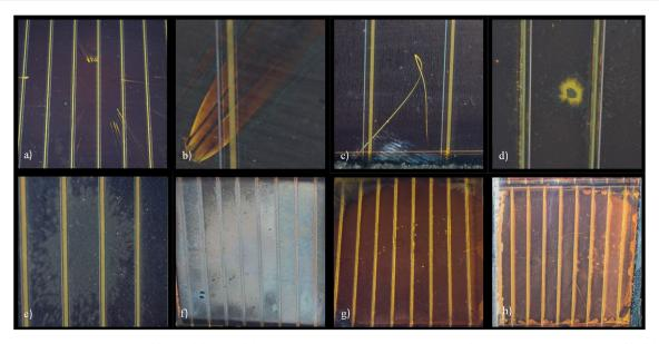
Fig. 2 GRAPE panels visual defects (a) and (b) flairs, (c) cracks, (d) holes, regions suffered by (e) oxygen penetration, and (f)-(h) moisture penetration in the panel module.
