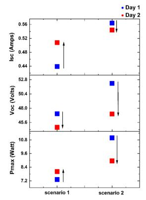
Fig. 9 Direct comparison of electrical characteristics for two consecutive days showcasing the two behavioral scenarios of the GRAPE panels.
