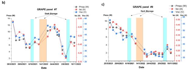
Fig. 4 Electrical parameters ( $P_{\text{max}}$ ,  $I_{\text{sc}}$ , and  $V_{\text{oc}}$ ) extracted from the I-V characteristics of (a) solar farm, (b) GRAPE panel #7, and (c) GRAPE panel #9 for the period 2021-2022. In graphs a, b and c, dark storage periods are highlighted with (a) cyan (1 month DS period applied twice), (b) orange (3 month DS period applied once).
