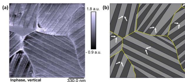
**Fig. 3** (a) Piezo-response force micrographs and (b) the anticipated ferroelectric domain polarization used in the DD model as a representative of the multi-grain surface section. Reproduced from ref. 46, copyright (2018), with permission from Elsevier.
