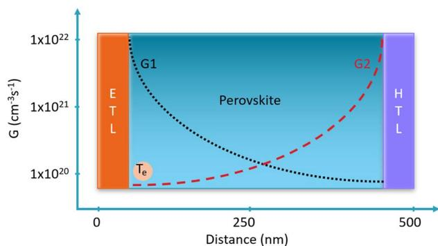
Fig. 5 Charge carrier generation profiles and electron traps in a perovskite solar cell.  $T_e$  represents an electron trap near the perovskite/ETL interface.  $G_1$  and  $G_2$  represent generation profiles upon light irradiance from the ETL and HTL sides, respectively.
